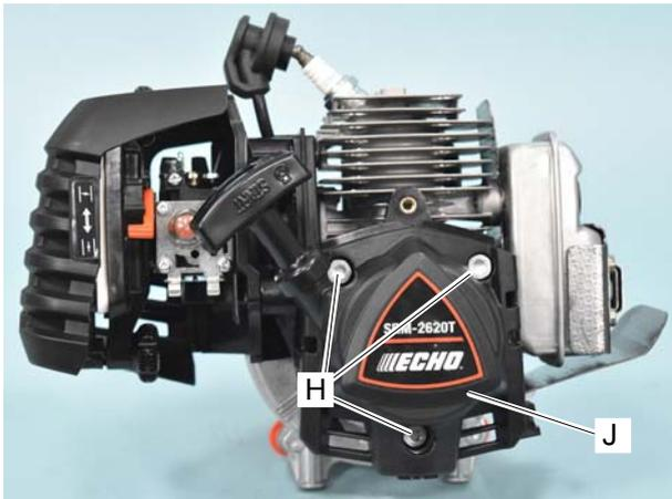
4. Remove bolts (H) and starter assembly (J) from unit.
