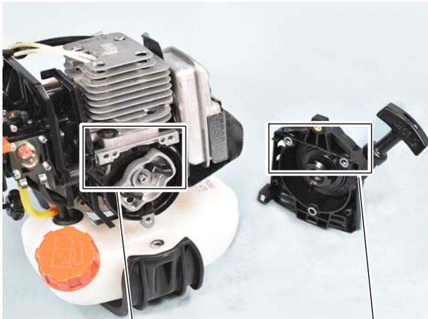
**NOTE:** Insert rib (h) of starter case to gap (f) between crankcase and dust cover. Insert rib (j1) of starter case to hole (g1) of crankcase. Insert rib (j2) of starter case to hole (g2) of crankcase as shown.
