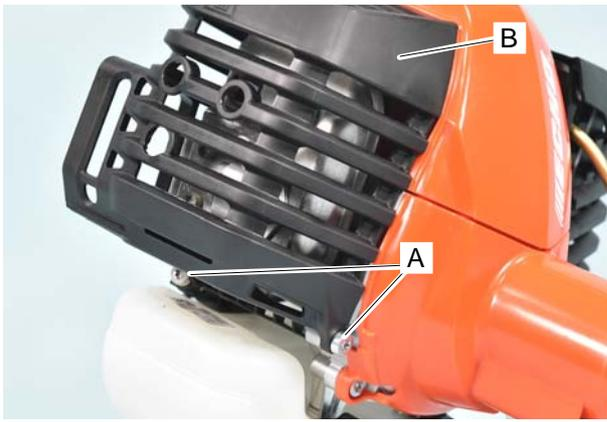
1. Remove bolts (A) and muffler cover (B).
