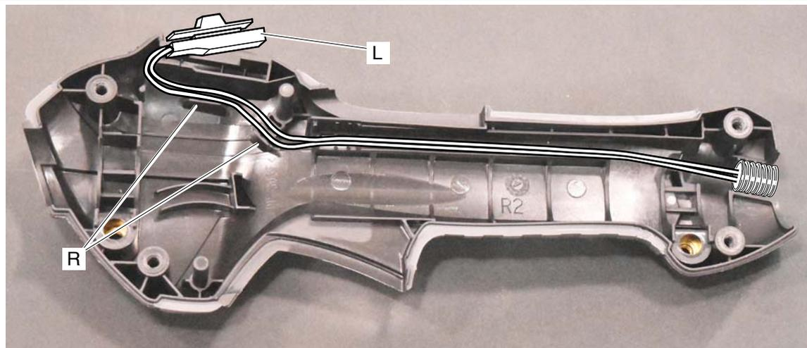
9. Route leads behind ignition switch (L), and then install ignition switch to rear handle grip half. Route leads through grooves and ribs (R) of rear handle grip half as shown.
