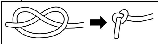
5. Pass the other end of starter rope through rope guide on starter case, then pass starter rope through starter grip and clip (B). Make a knot as shown.
