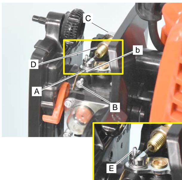
1. Confirm throttle plate (A) contacts tip (b) of throttle adjust screw (B) when throttle trigger is in idling position.
