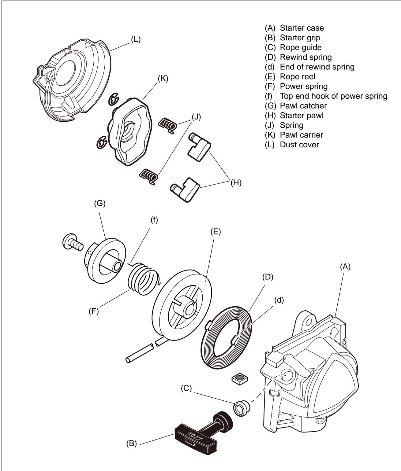
2-1 Disassembling starter assembly
