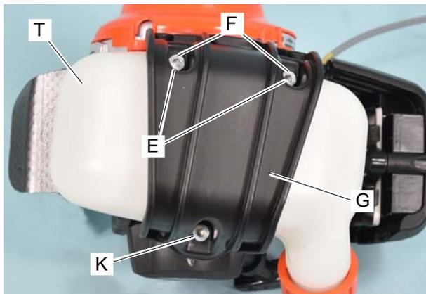
3. Remove bolts (E), washers (F) and bolt (K) under fuel tank.
