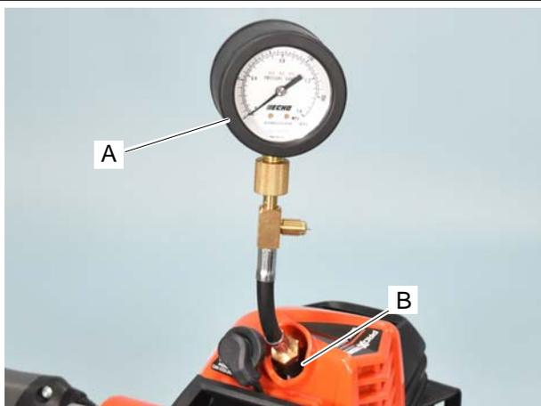
**NOTE:** Test cylinder compression when engine is cold.
