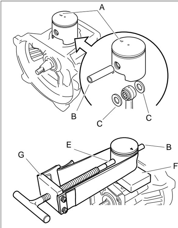
1. Place piston over the small end of connecting rod, so that the arrow mark (A) on piston points toward muffler.
