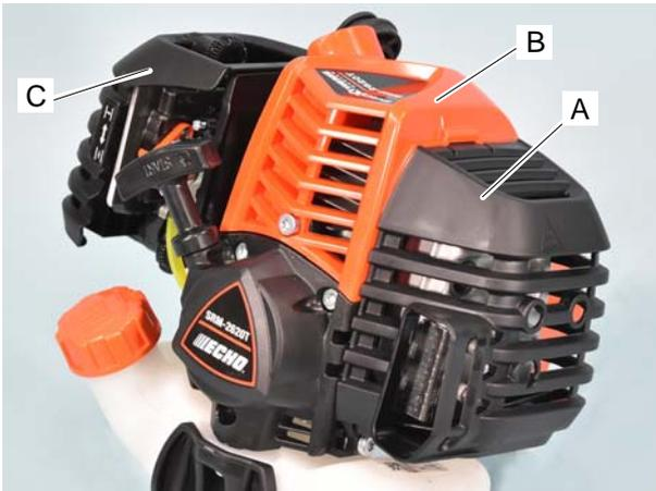
1. Inspect muffer cover (A). If blocked with leaves or other debris, clean out debris as required.
