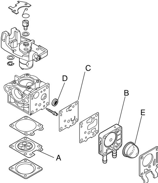
1. Check metering diaphragm (A) for hardening, distortion or pin hole. Replace it as required.
