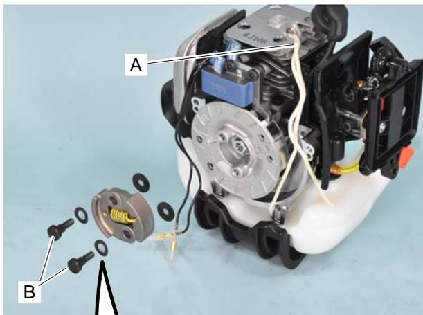
1. Pre-assemble clutch hub, clutch shoes and springs.
