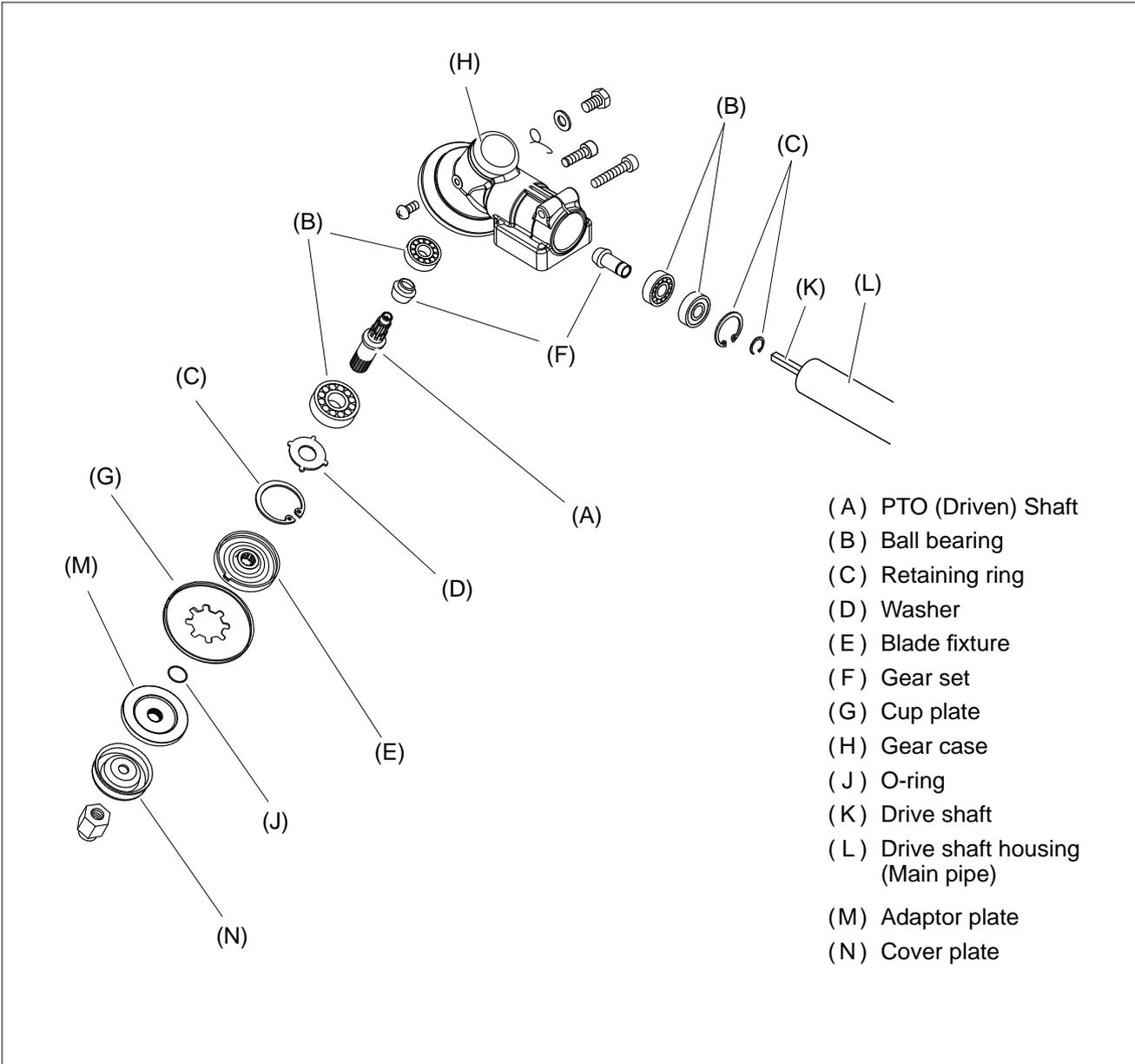
7 CUTTER DRIVE SYSTEM on SRM-2620TES, C262TS and T262TXS
