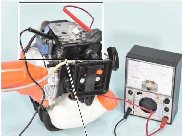
1. Connect one probe of Ohm-meter or multimeter to spark plug cap coil (A).
