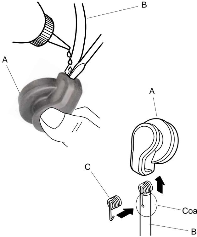
1. Disconnect spark plug cap (A) from spark plug.
