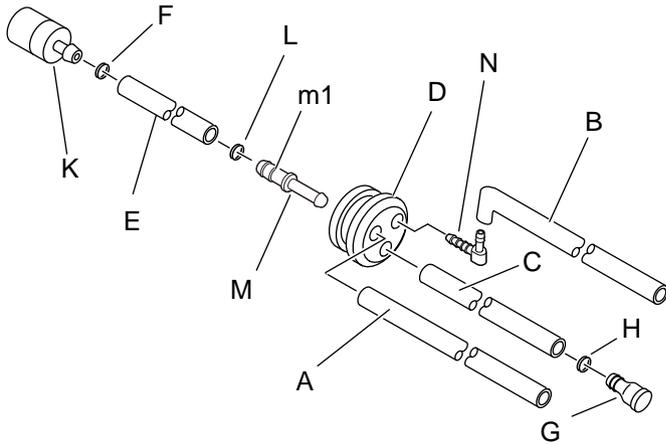
5. Set clip (F) on fuel line (E) and connect fuel strainer (K) as shown.
