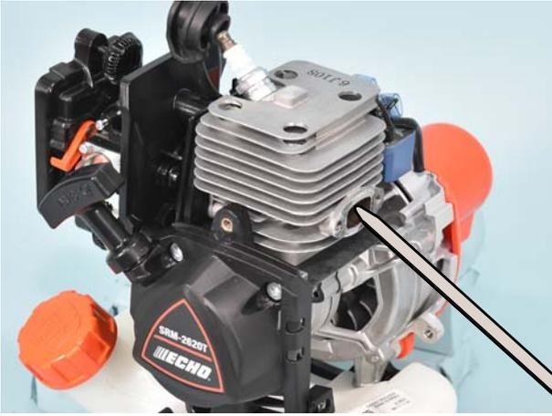
1. Remove muffler cover and cylinder cover.
