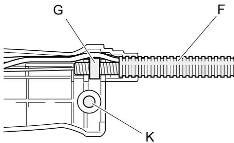
12. Seat square nut (G) in dent of handle grip and push in corrugated tube (F) to the grip two or three grooves from tube end.
