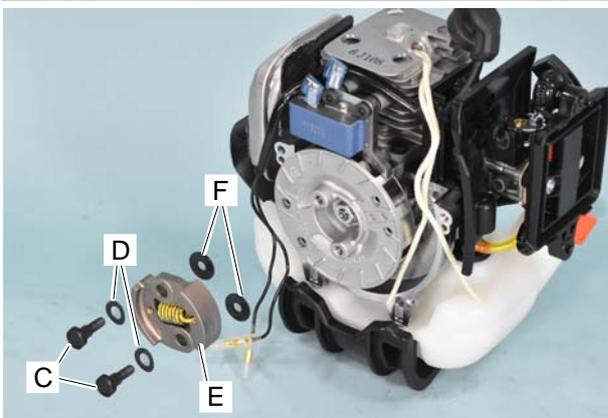
5. Remove bolts (C), spring washers (D), clutch shoe (E) and washers (F).
