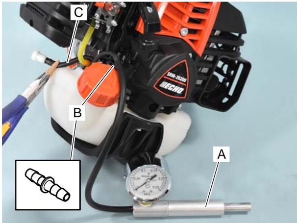
1. Remove air cleaner cover. Disconnect black fuel line from carburetor and connect pressure tester 897803-30133 (A) to fuel line with joint pipe V186-000150 (B).
