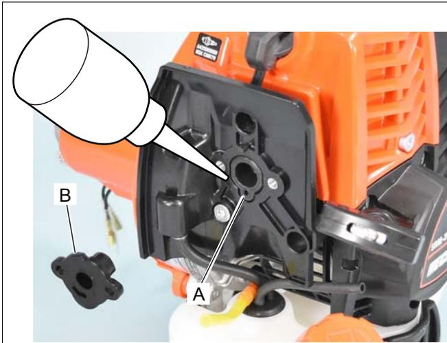
1. Remove carburetor and insulator plate boot (B), and drop a little oil in pulse hole (A) on intake bellows.
