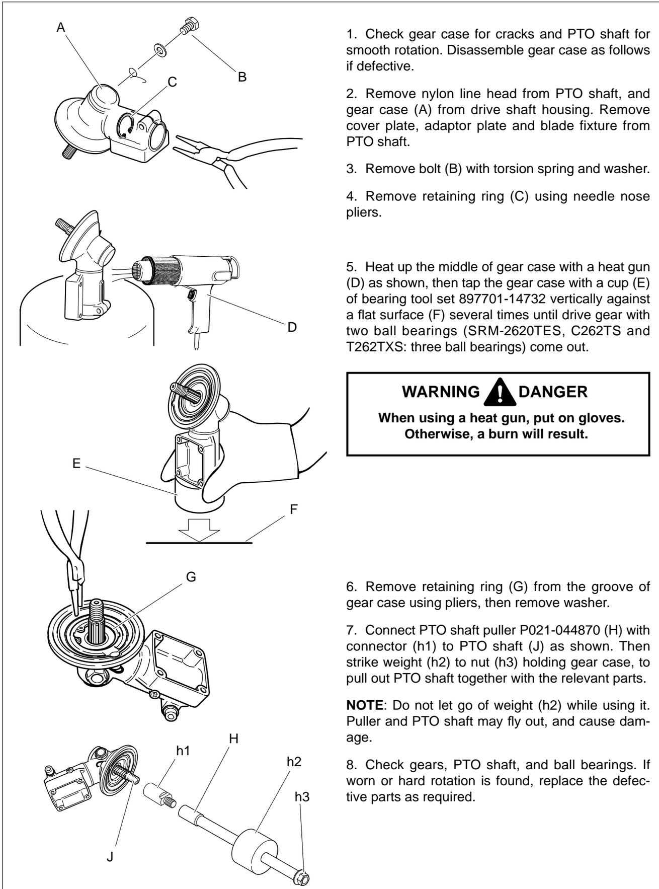
1. Check gear case for cracks and PTO shaft for smooth rotation. Disassemble gear case as follows if defective.
