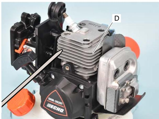
3. Inspect cylinder cooling fins (D) for blockage with dirt or dust.
