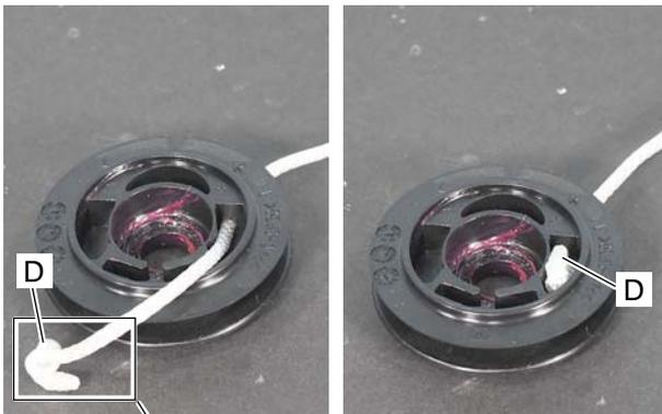
4. Make a knot (D) at end of starter rope and pass the starter rope through hole of rope reel, then press the knot (D) into reel well as shown.
