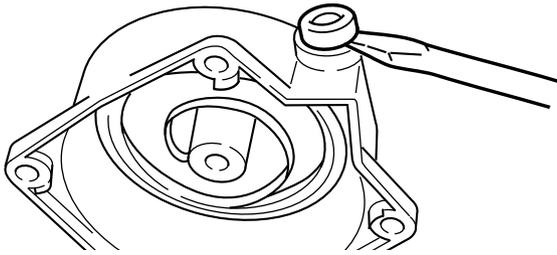
If rope guide is worn out or damaged, replace it as follows:
