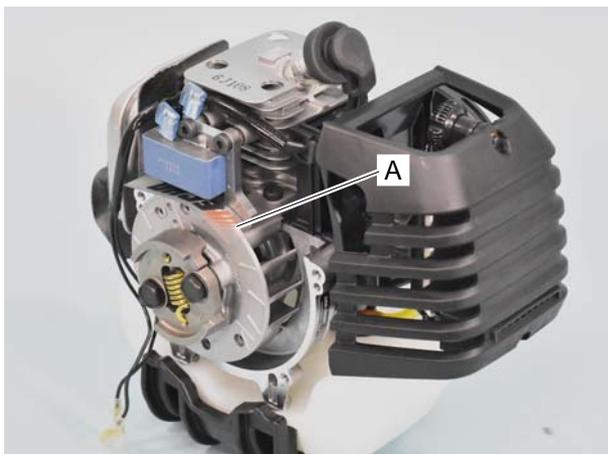
1. Insert Module air gap gauge: 91004 (A) or 0.3 - 0.4 mm (0.012 - 0.016 in) thick feeler gauge between flywheel and ignition coil shoes.
