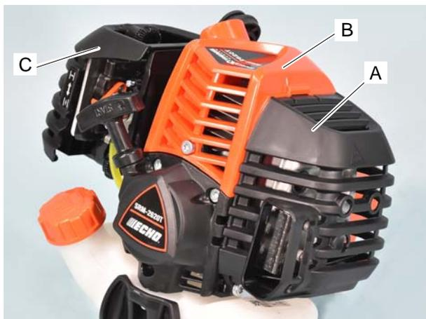
1. Inspect muffler cover (A). If blocked with leaves or other debris, clean out debris as required.
