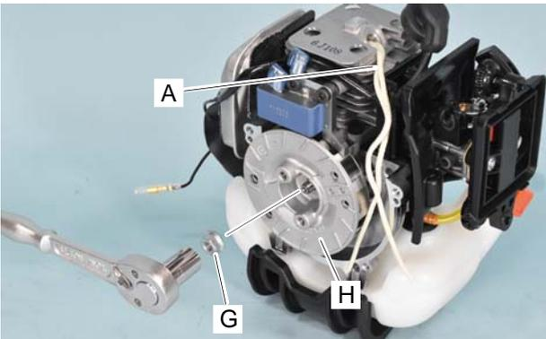
6. Remove flange nut (G) on flywheel (H) using 13 mm (0.51 in) box wrench (B) or similar tool.
