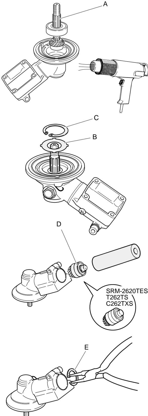
1. Heat up the top of gear case with a heat gun as shown, then insert the assembled PTO shaft (A) into gear case until its bottom.
