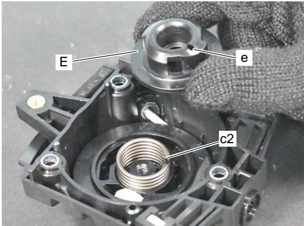
4. Install pawl catcher, assembling power spring hook (c2) into hole (e) of pawl catcher (E).
