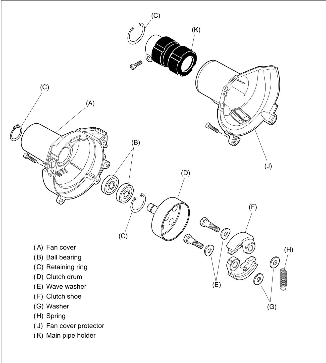
5-1 Removing clutch shoes and springs
