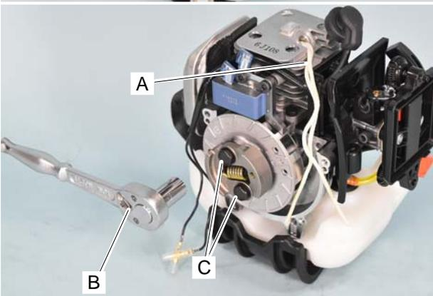
3. Install rope (A) into spark plug hole by hand, to stop crankshaft rotation.
