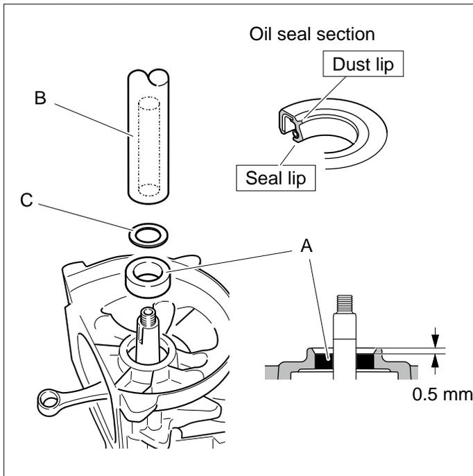
1. Pry defective oil seal from engine.
