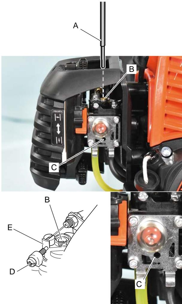
Tools Required : Small screwdriver with 2.5 mm blade, P/N G310-000050 electronic tachometer, P/N Y089-000094(A) small D-shaped tool.
