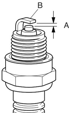
1. Remove spark plug to inspect for fouling, cracked or broken insulator, or rounded center electrode. Clean or replace spark plug as required.
