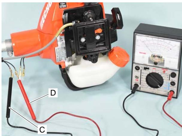
3. Connect one probe of Ohm-meter or multi-meter to primary lead (C) of ignition switch side as shown.
