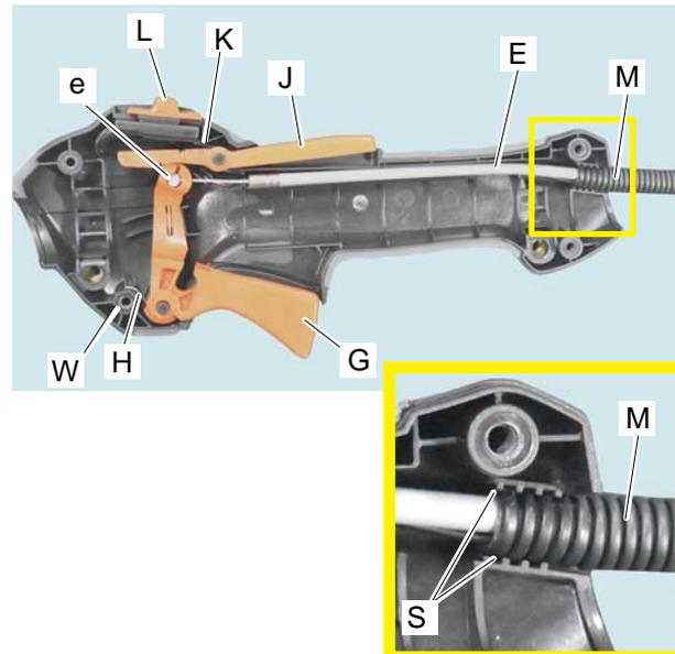
12. Connect end (e) of throttle cable (E) to throttle trigger (G). Install throttle trigger (G), hooking torsion spring (H) on the post (W) as shown.
