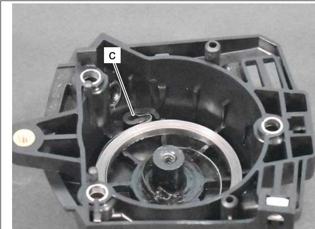
Rewind spring supplied as spare part is shipped in temporary retainer.
