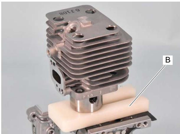
**NOTE:** When installing cylinder, it is convenient to use piston holder 897719-02830 (B) for stabilizing piston.
