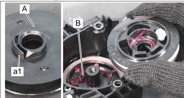
**NOTE:** Apply Lithium based grease in starter case.
