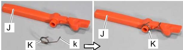
11. Set torsion spring (K) to throttle lockout lever (J) as shown.
