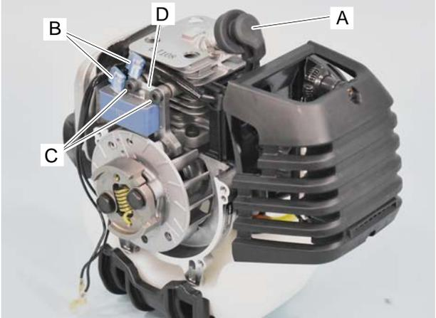
1. Disconnect spark plug cap (A) from spark plug.
