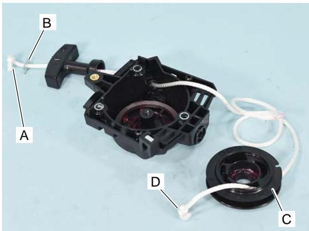
1. Pull out knot (A) and clip (B). Untie knot (A).
