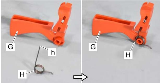
10. Set torsion spring (H) to throttle trigger (G) as shown.
