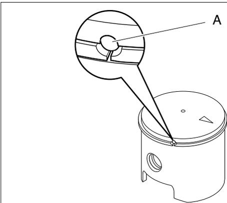
1. Install piston ring on piston, ensuring the end gaps of piston ring are properly positioned around locating pin (A) as shown.
