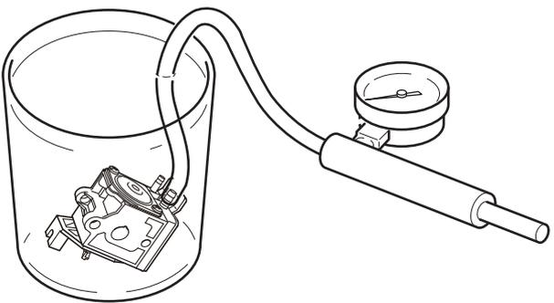
1. Remove air cleaner cover. Push purge bulb several times to fill and wet fuel pump circuit with fuel.
