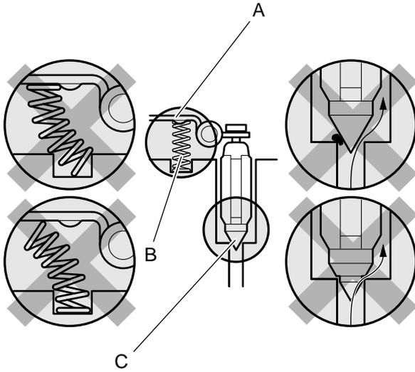
1. Remove metering lever (A) and pivot pin. Remove spring (B) and inlet needle valve (C).
