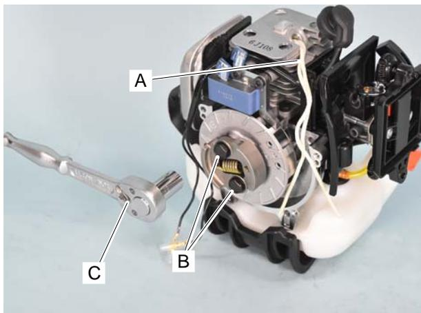
1. Remove muffler cover, engine cover and fan cover.
