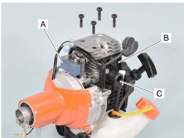
1. Remove cylinder from engine.
