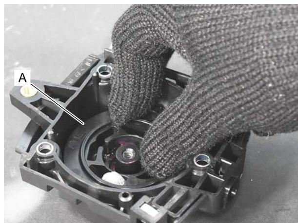
2. Check for proper engagement of rewind spring and rope reel by turning rope reel (A) clockwise and counterclockwise.
