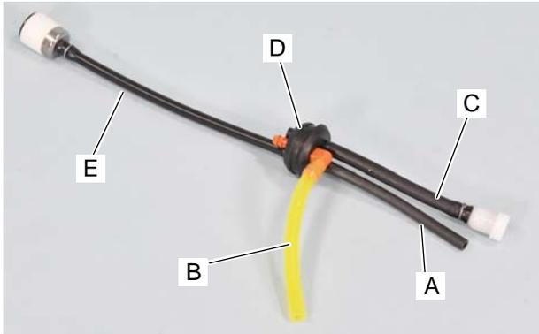
1. Disconnect fuel line (A) and fuel return line (B) from carburetor.
