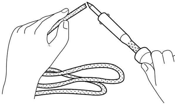
3. When installing a new starter rope, singe both ends of the rope to prevent from fraying.
