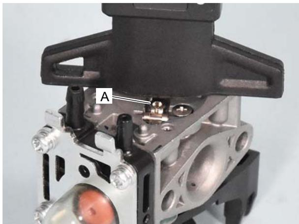
1. Remove metering diaphragm cover, metering diaphragm and gasket.
