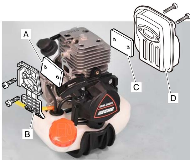
1. Remove cylinder cover, muffler, air cleaner cover and carburetor.
