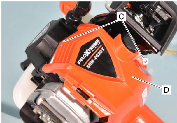
2. Remove bolts (C) and cylinder cover (D).
