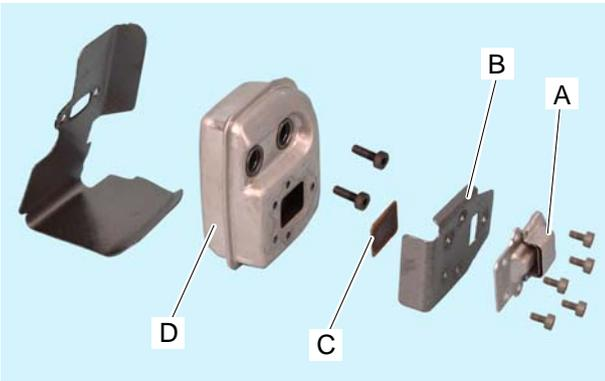
4. Remove exhaust guide (A), exhaust gasket (B) and spark arrester screen (C) from muffler (D).
