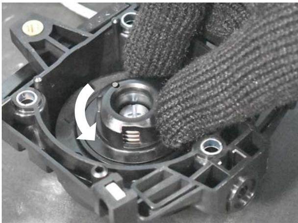
7. Pull starter several times to check rewind spring tension. If starter is not rewinding fully, rotate rope reel one more turn counterclockwise following above step (6).
