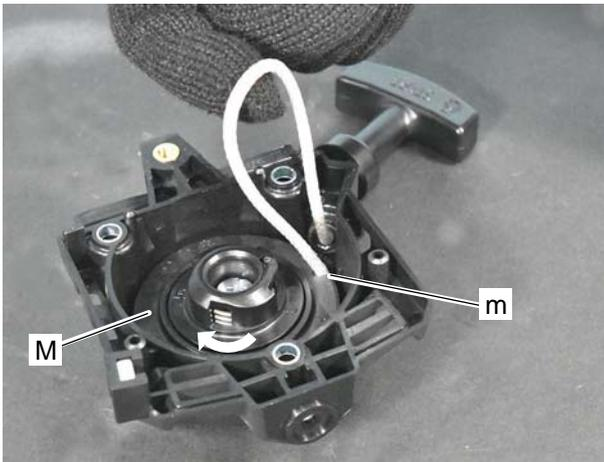
5. Pull out starter rope about 30 cm (12 in) and hold rope reel (M) by hand. Loop excess rope in rope reel notch (m) as shown.
