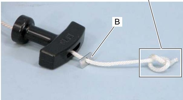
6. Tighten knot. Push knot in starter grip with clip (B).
