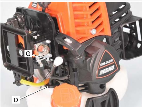
12. Install grommet (D) with lines and fuel strainer to fuel tank as shown.
