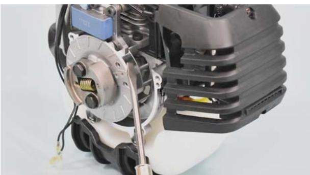
1. Inspect magnetic force of flywheel using flux meter, or bridging with a screwdriver as shown.
