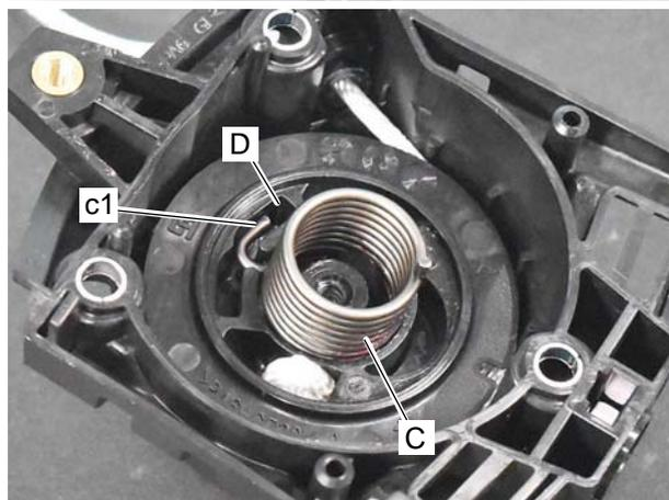
3. Install power spring (C) assembling hook (c1) of power spring into rope reel well (D).
