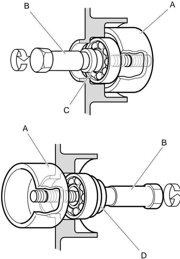
1. Check main ball bearing for smooth rotation, after disassembling crankshaft. If rough, replace it (them) with new one.
