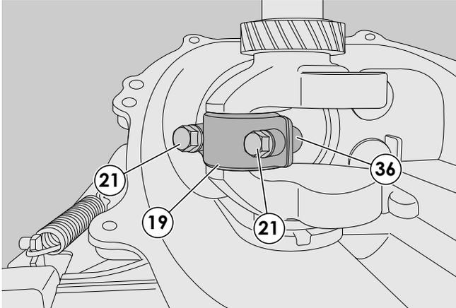
23 - Mount the engine shaft (24) and the connecting rod cap (19) with the relative screws (21), taking care with the position references (36) so as to avoid inverting the mounting direction of the cap.
