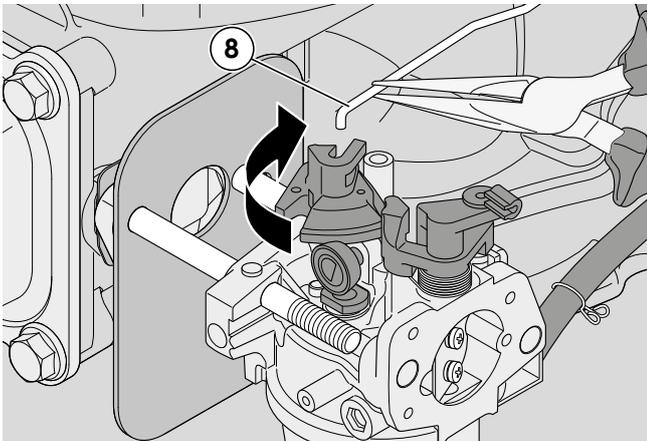
7 - Rotate the butterfly valve clockwise 90° and, using pliers, disconnect the intake butterfly rod (8).
