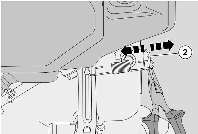
2 - Using pliers, bend the plate (2) slightly to the right to increase the number of revs and to the left to reduce them.
