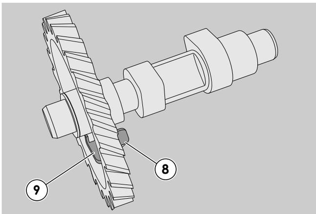
6 - Check the regular movement of the pressure reducer (8) and the efficiency of the spring (9); the whole group must always be replaced in the case of breakage or irregular operation of the pressure reducer.
