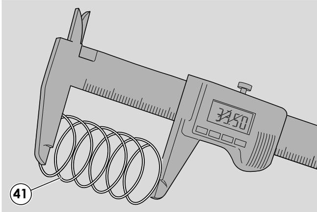
6 - Check the free length of the spring (41) and replace the spring if it is less than 33,50 mm.
