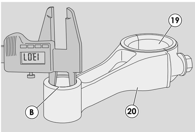
16 - Fit the cap (**19**) to the connecting rod (**20**) and check the diameter from the gudgeon pin side and the crank side; replace the connecting rod if the values are greater than:
