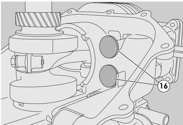
11 - Before fitting the camshaft ensure that the two tappets (16) are correctly housed in their seats.
