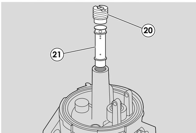
11 - Undo the main jet (20) and pull out the pilot jet (21).
