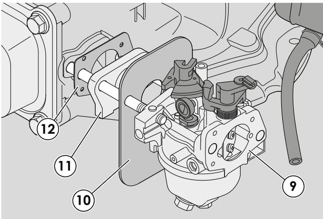
8 - Completely remove the carburettor (9) the gasket (10), the spacer (11) and the heat protection gasket (12).
