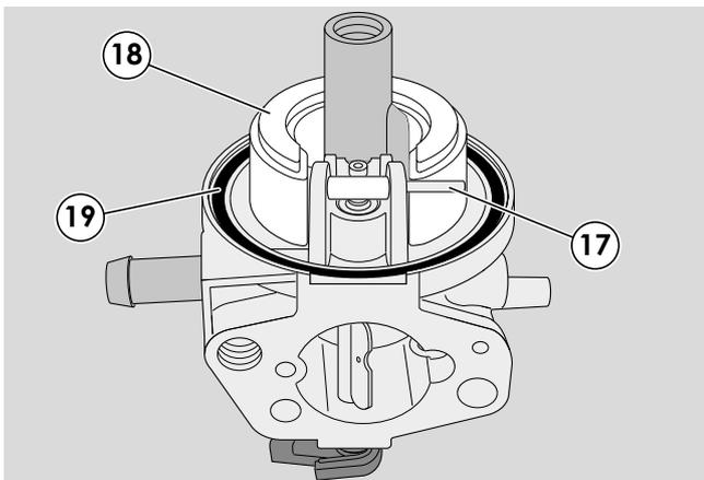
10 - Pull out the pin (17), dismount the float (18) and remove the gasket (19).
