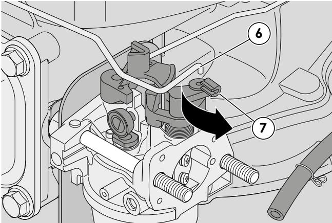
6 - Remove the tie rod (6) of the AUTO-CHOKE lever by releasing the locking clip (7). Slightly pull out the carburettor to facilitate the release of the intake butterfly shaft.
