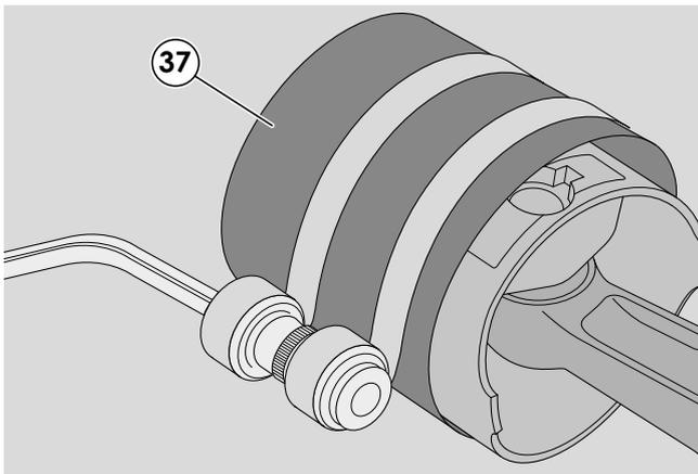
22 - Oil the inside of the piston liberally and insert the piston, with the marking facing the exhaust.
