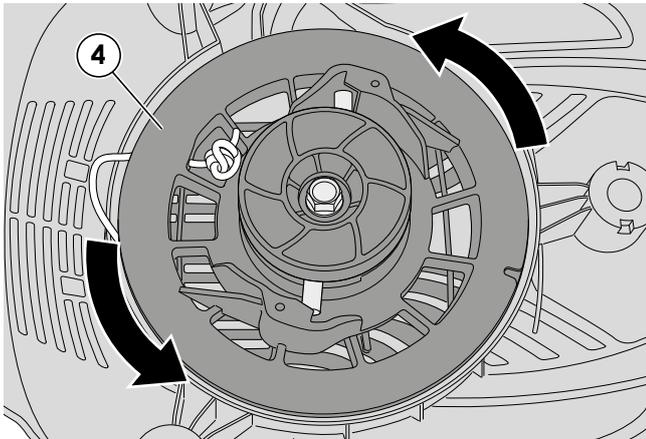
4 - Rotate the pulley (4) through about 7 complete turns anticlockwise in order to load the spring and hold it still.
