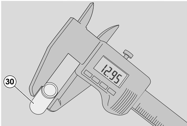
14 - Check the diameter of the gudgeon pin (**30**) in several places and replace it if it is less than 12.95 mm, even at a single point.
