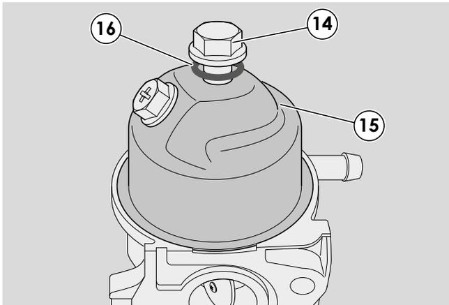
9 - Unscrew the central screw (14) securing the tank (15) and remove the corresponding OR (16).
