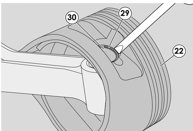
13 - Use a screwdriver to remove the clamping ring (29) and remove the gudgeon pin (30) from the piston (22).
