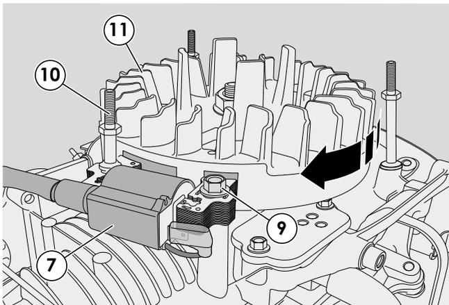
4 - Slack off the screw (9) and the stud (10) which secure the coil (7).
