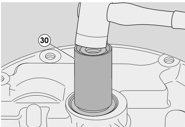
4 - Complete the insertion with the help of a pipe (30) of a diameter of approximately 30-35 mm.
