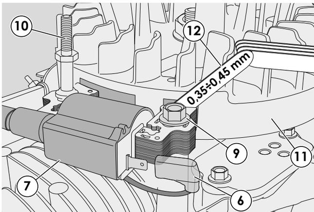
5 - Insert a 0,35 mm thickness gauge (12) between the complete flywheel (11) and the coil poles (7), push the coil until the poles come in contact with the thickness gauge and secure screw (9) and stud (10); with the flywheel locked, the airgap must be between 0,35 and 0,45 mm.
