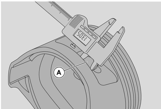
15 - Check the diameters of the gudgeon pin housings (**A**) on the piston (**22**) and replace the piston if they are more than 13.05 mm, even at a single point.
