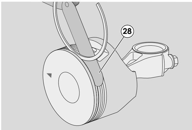
12 - To check the wear in the piston ring housings, fit a new ring and measure the residual space with a feeler gauge (28). The piston must be replaced if it is greater than 0.15 mm in the two compression ring housings.
