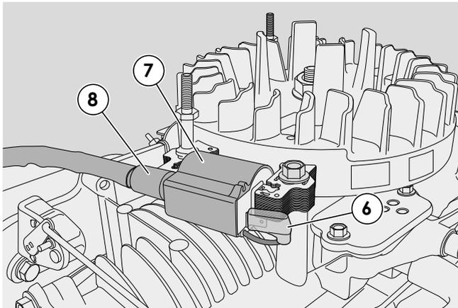
1 - Remove the starter assembly [
