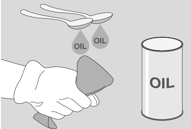
**!** **WARNING:** The filter elements must be kept well cleaned and soaked in oil. Replace them if broken, cut or with crumbled parts. Do not use compressed air to clean the filters.
