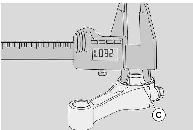
If the connecting engine shaft is outside measurement tolerances or has small scratches or marks, it is necessary to replace it.
