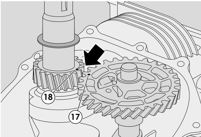
24 - After having fixed the connecting rod cap, take the greatest care to ensure that the two position references (17) and (18) punched on the engine shaft and camshaft gears, coincide, ensuring the correct distribution phasing.
