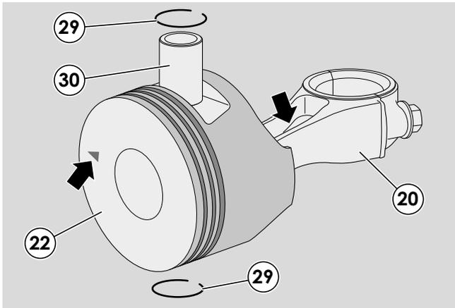
20 - Fit the connecting rod (20), gudgeon pin (30) and clamping rings (29) to the piston (22).
