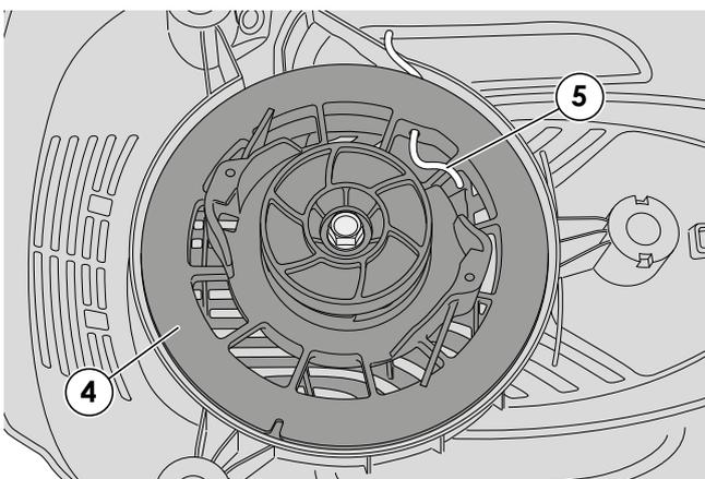
3 - Undo or cut the knot at the end of the rope (5) and remove the section still attached to the pulley.
