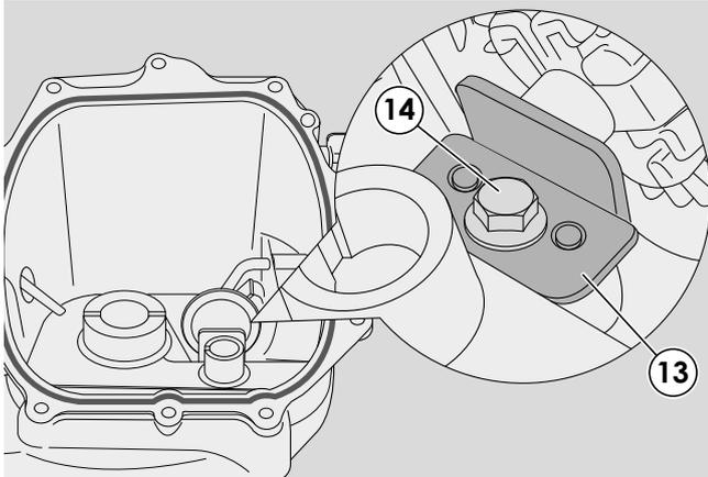
9 - In the case of breakage or irregular operation of the counterweights the whole group, fixed by a plate (13) and a screw (14) must be replaced.
