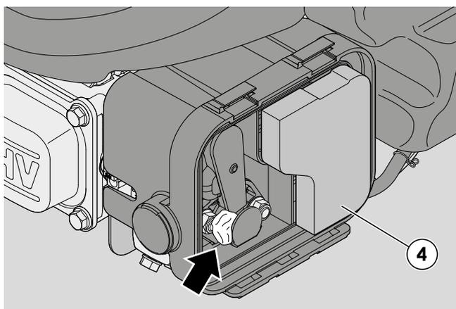
5 - Check carefully that the filters are not damaged. If they are, replace them.
