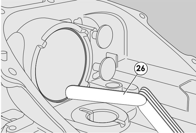
10 - To check the wear in the compression rings, insert them one at a time into the cylinder (23) by about 10-15 mm and measure the gap between the two ends with a feeler gauge (26); the rings must be replaced if the gap is more than 1,0 mm.
