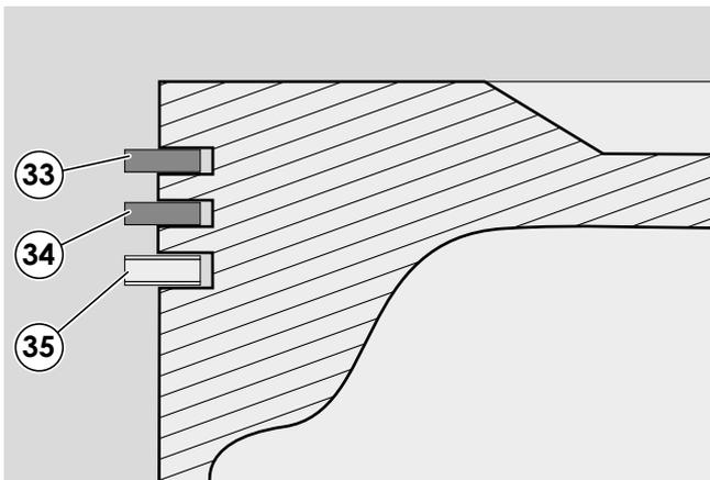
19 - To refit the rings to the piston, first fit the three oil scraper rings (33), then the ring with a round edge (34) and finally the ring with a sharp edge (35), being careful over the markings (which must face the piston head) and in arranging the gaps to ensure that they are not aligned with each other;
