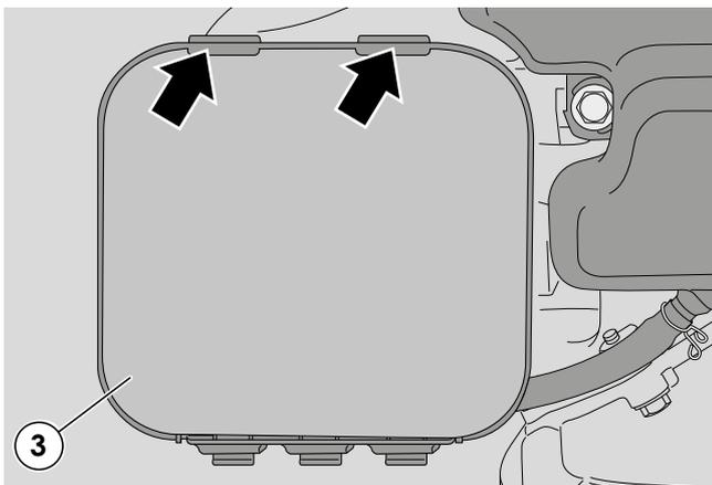
**!** **WARNING:** When assembling the filter element (3), make sure it is properly positioned between the tabs, as shown in the figure.
