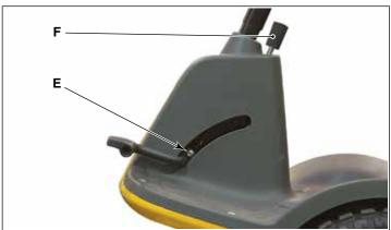
3. Remove the lift pedal, screw (E). Also remove the plastic knob (F) by pulling it straight up.
