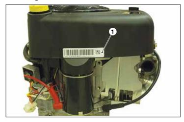
The engine is built to precise technical specifications which distinguish it from similar products made by the same manufacturer. The serial number indicated on the label (1) makes it possible to correctly identify the product and its characteristics and must always be cited when ordering spare parts or requesting any information from the Manufacturer.
