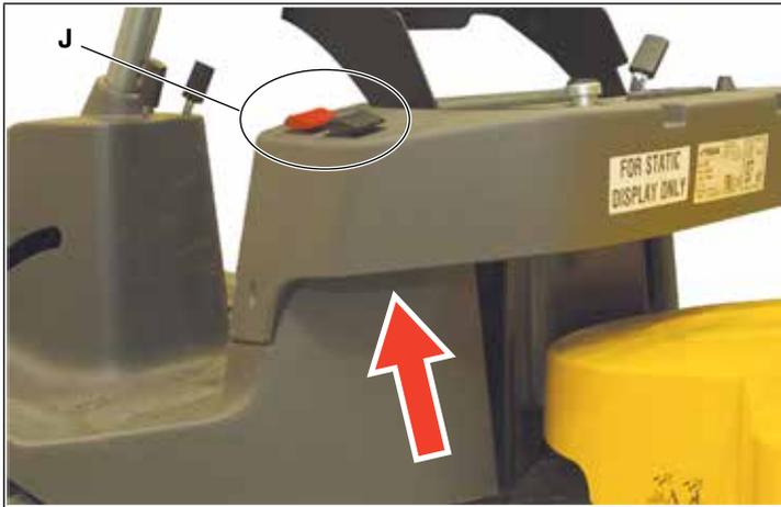
6. Remove the fruits from the switches (J) by operating from under the covering;
