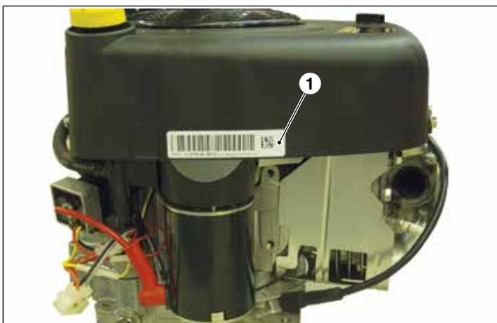
The engine is built to precise technical specifications which distinguish it from similar products made by the same manufacturer. The serial number indicated on the label (1) makes it possible to correctly identify the product and its characteristics and must always be cited when ordering spare parts or requesting any information from the Manufacturer.
