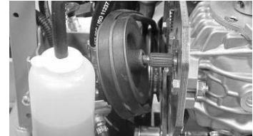
8. Remove the M10 screws G (3x) that hold the carrier plate/pulley to the flywheel as follows:
