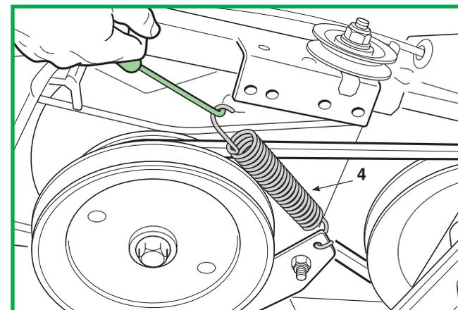
Disconnect the spring (4) and move the tightener (5) so as to release the belt (6) from the pulley (7).
