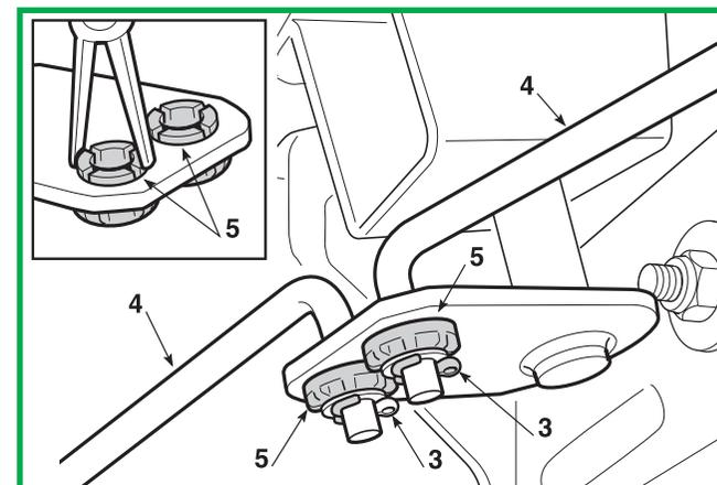
If the bushes (5) should need replacing due to excessive play, they can be extracted using pliers.
