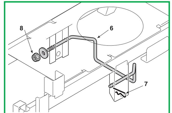
Disassemble the belt guide blade (6), fixed by a cotter pin (7) from the left side and by a nut (8) from the right.
