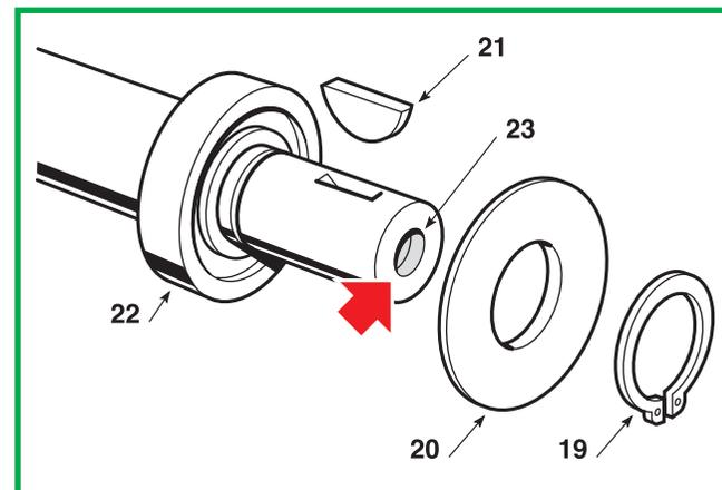
The second bearing still in place must be removed by hitting it from the inside of the flange using a 12 ÷ 15 mm diameter round bar (24).
