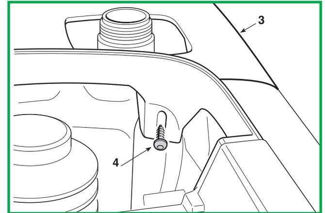
**NOTE** - Removing the rear part (3) is facilitated by widening the two side elements slightly and lifting the rear part just enough to disconnect the three fins (7).
