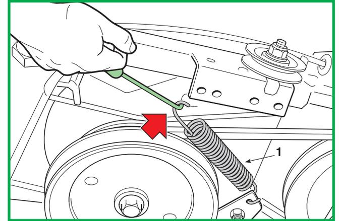
Unhook the drive belt tightener spring (1).
