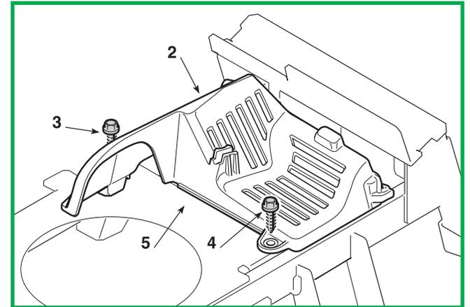
Remove the guard (2), fixed by a screw (3) from the right and by a screw (4) from the left.
