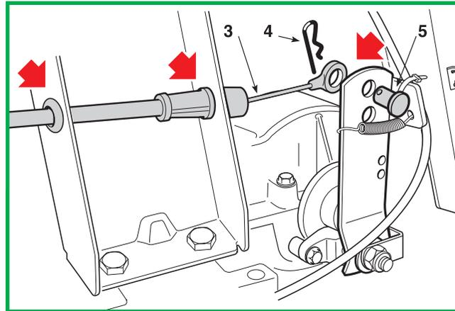
When mounting, restore the cable route (3) following layout instructions, making sure you replace the clamp (6).
