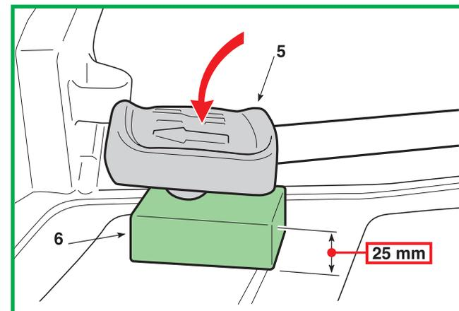
This is obtained by placing a block (6) under the pedal (5) and working on the nuts (7) until the desired situation is reached. Taking care not to change the position of the lever (3) by mistake during adjustment.
