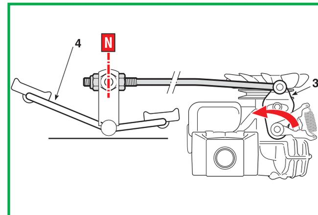
To reach the forward and reverse speeds set (thus establish the pedal's “neutral” position), the edge of the reverse gear pedal (5) at rest must be 25 mm from the footplate with the hydrostatic group lever (3) on “neutral”.
