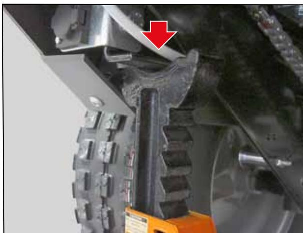
– Stabilize the machine with two stands placed in correspondence of load-bearing elements of the front part of the frame.
