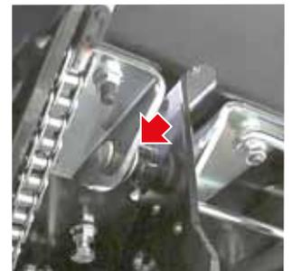
In the case of hardening when operating the pedal, a practical test consists in disconnecting the pedal lever from the linkage; if the pedal movement regains normal smoothness and quickly returns to the central position, it means that the cable must be replaced.
