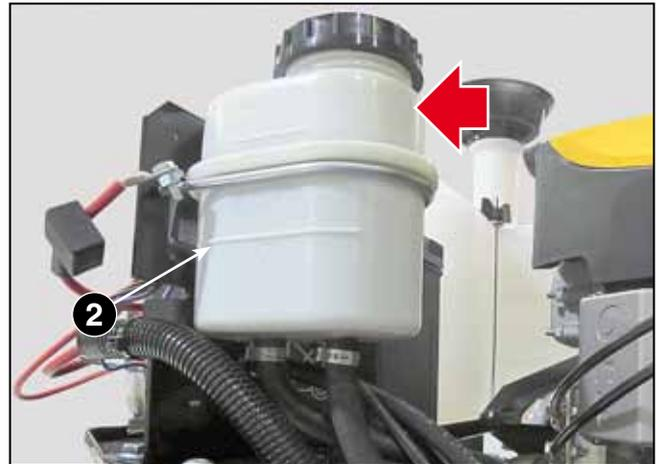
**IMPORTANT** *The topping up operation may also be necessary during the purging phase; it is always necessary to avoid that the tank remains empty and the system sucks air. This could result in damage to the transmission components. Frequently check the oil level and top up from the cap (1) of the tank (2), whenever it's necessary to restore the level.*
