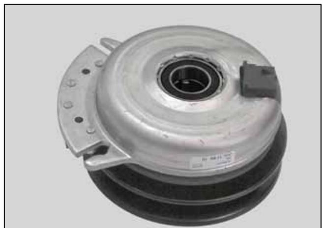
The clutch is engaged by applying current to the coil connection. This results in a current flowing through the coil, magnetizing the coil pulling the armature onto the rotor with sufficient force to hold the two pieces together, connecting the output and the input shafts firmly together. The force of the armature against the rotor pulls it away from the brake, hence releasing the brake.
