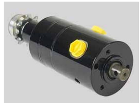
The steering unit is connected to the steering wheel via the steering column. During the steering, the steering wheel moves a gear that has an orbital movement with respect to the external toothed gear. Inside the steering unit, the rotor, which acts as a volumetric dispenser, releases a quantity of oil proportional to the steering angle made by the steering wheel.
