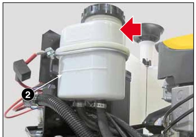
10. Check that the oil level in the tank (2) has reached the correct level.
