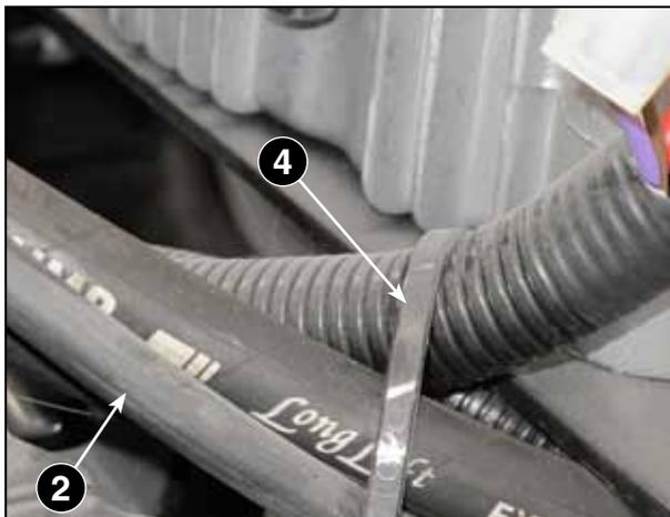
2. Cut the clamp (4) to ease the extraction of the cable (2).
