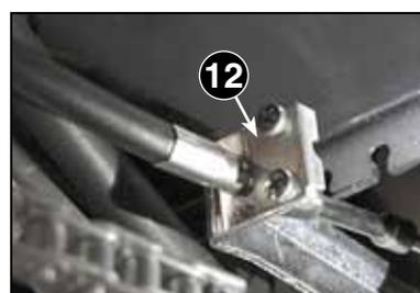
6. Unscrew the two screws (13), remove the plate (12) and release the cable (6) from the ring of the support bracket (14).
