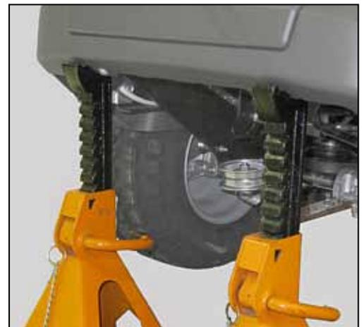
– Stabilize the machine with two stands placed in correspondence of load-bearing elements of the front part of the frame.
