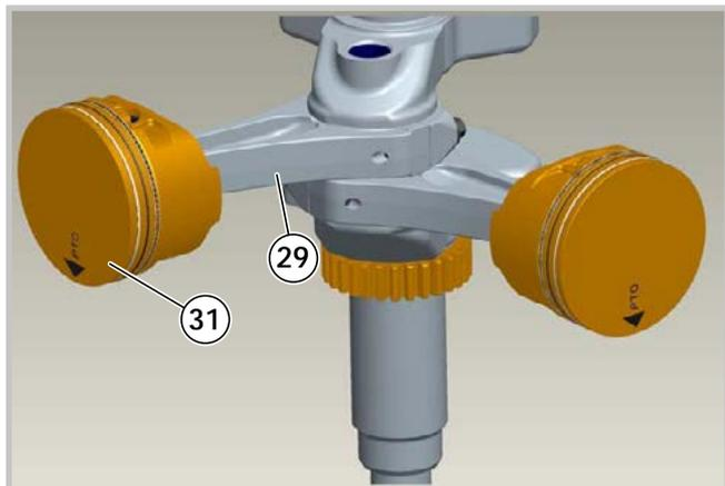
22 - Fit the connecting rod (29), gudgeon pin and clamping rings to the piston (31).
