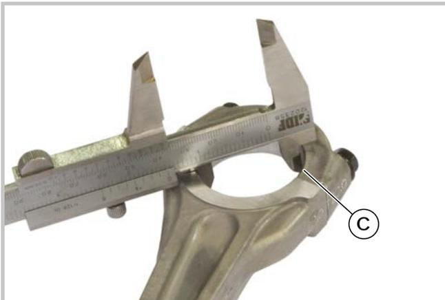
If the connecting rod is outside measurement tolerances or has small scratches or marks, it is necessary to replace it.
