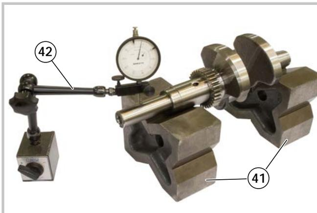
20 - To check the alignment between the manifolds and the protruding part of the shaft, place the engine shaft on two prismatic guides (41) and, with the help of a comparator (42) placed at the end, check the displacement by rotating the shaft. The shaft must be replaced if the displacement exceeds 0,10 mm.
