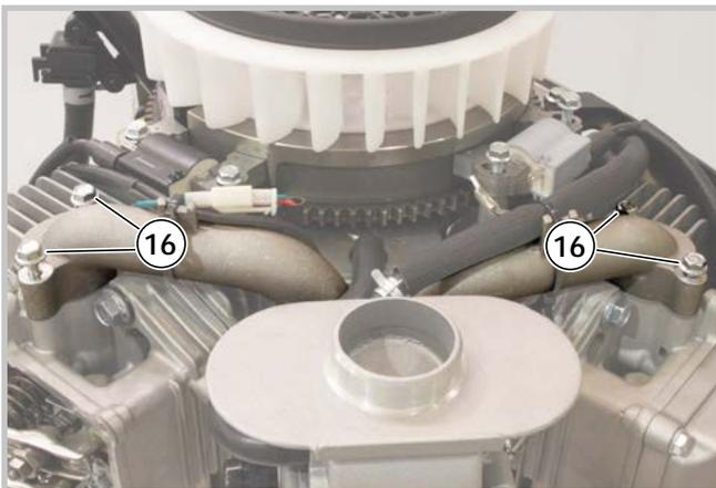
3 - Remove the four screws (16) present in torque in the two carburettor manifolds.
