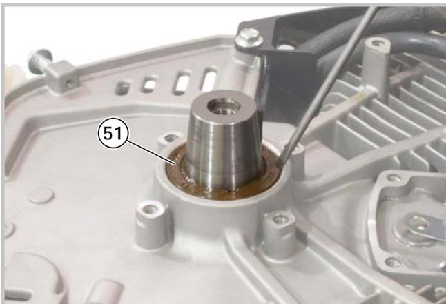
4 - Use a thin screwdriver inserted under the sealing lip to extract the oil seal ring (51).
