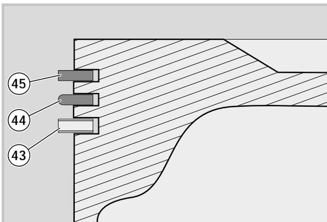
21 - To reassemble the segments on the piston perform sequentially:
