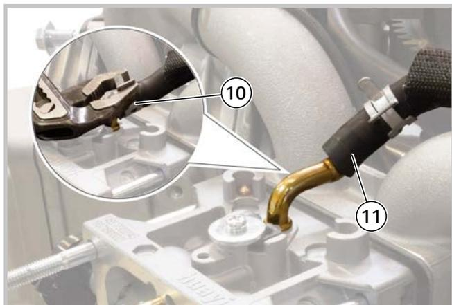
5 - Using plier, remove the clamp (10) and disconnect the petrol hose (11). Collect all the fuel in the tank and hose in a suitable container.
