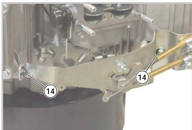
7 - Operate the steering lever, loosening the fixing nut on the right (14) and removing the one on the left (14).
