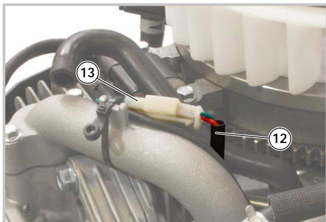
6 - Disconnect the connector (12) connected to the carburettor solenoid (13).
