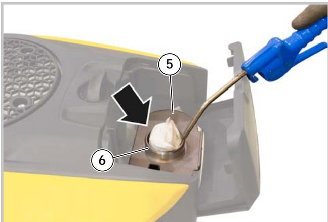
7 - With a jet of compressed air, clean inside the seat (5) of the filter by removing dust and remains of grass, making sure that the intake pipe hole (6) is closed so that nothing gets inside the pipe.
