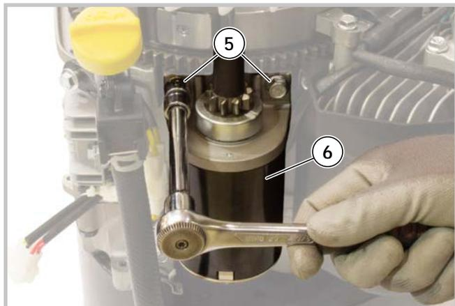
4 - Remove the two screws (5) and remove the starter motor (6).
