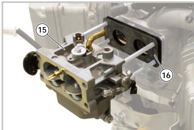
8 - Completely remove the carburettor (15) from its housing and the gauge (16) with the two gaskets.
