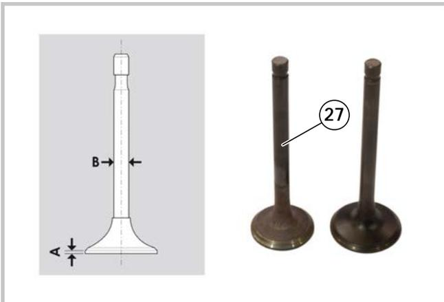
7 - Remove all incrustations from the valve head (27) with abrasive cloth and check the thickness of the margin (A); the valve must be replaced if the margin (A) is less than between 2,80 mm and 3,20 mm (inlet - IN/YI) or between 3,30 mm and 3,70 mm (exhaust - EX/YE) or if it shows signs of burning.
