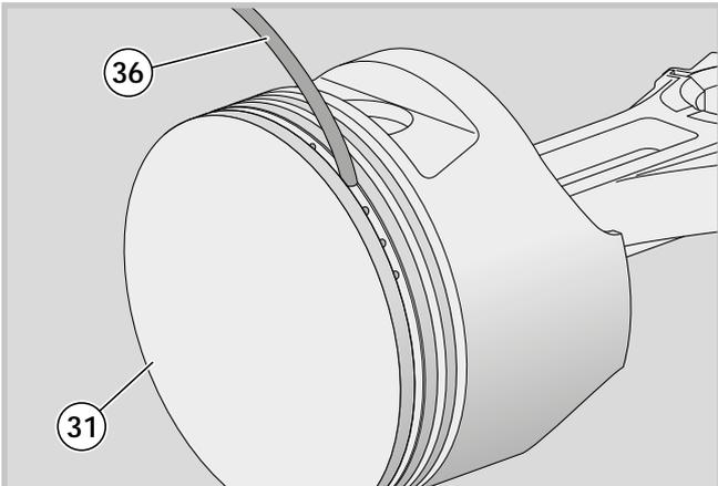
13 - Use a section of an old ring (36) to carefully clean the inside of the piston (31) ring housings, ensuring that the oil passage holes are not blocked.
