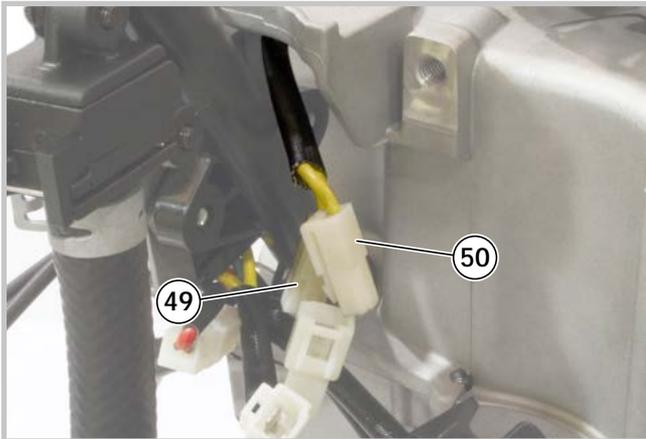
3 - Disconnect the two connectors (49) and (50) and remove the alternator (47) from the seat.
