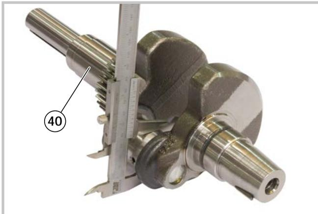
19 - Remove the engine shaft (40), checking the diameter of the connecting rod pin with a digital gauge. The value must not be less than 37,93 mm or the engine shaft will have to be replaced.
