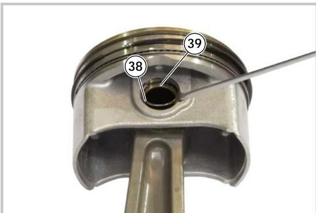
15 - Use a screwdriver to remove the clamping ring (38) and remove the gudgeon pin (39) from the piston (31).
