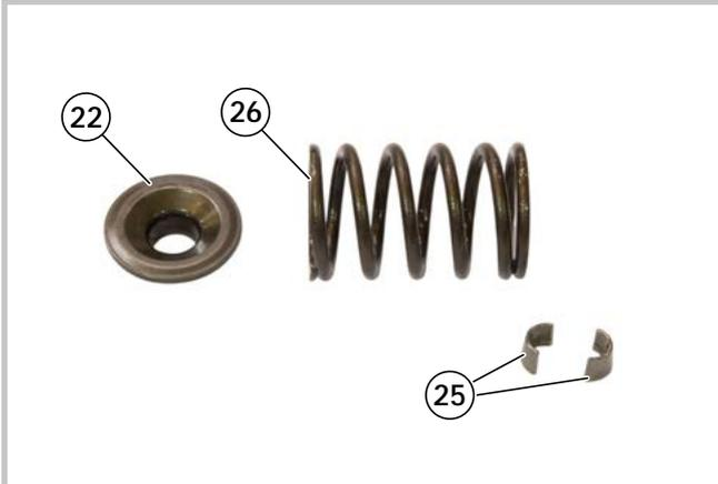
6 - Remove the cup-washer (22), the spring (26) and the two half-cones (25).
