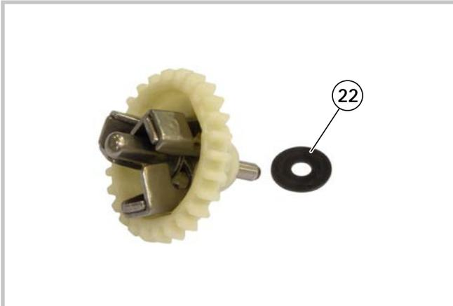
9 - In the case of breakage or irregular operation of the counterweights assembly; remove the centrifugal assembly, and retaining the shim washer (22).
