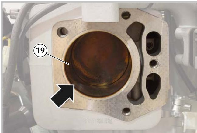
7 - Turn the flywheel manually to move the piston and clean inside the cylinder (19).
