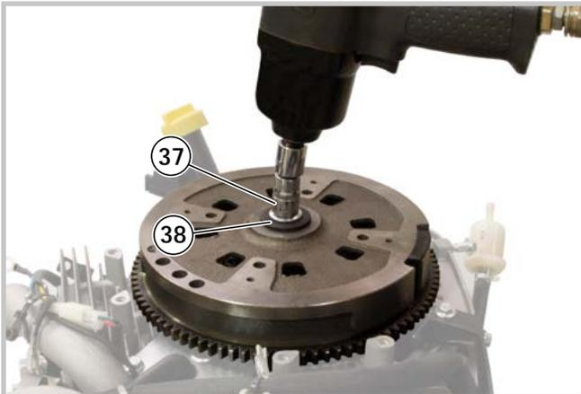
5 - Using a pneumatic gun, unscrew the nut (37) and recover the washer (38).
