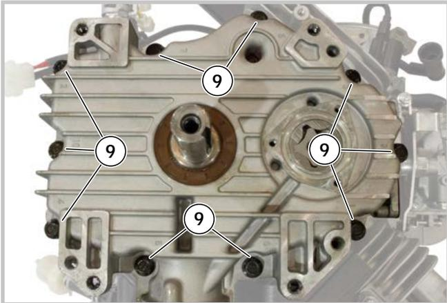
5 - Open the crankcase sump by unscrewing the ten screws (9).
