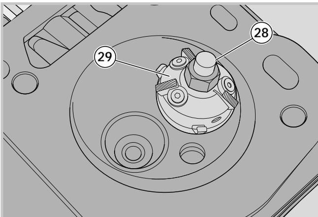
**NOTE - The valve seats must be ground by hand, using a special grinding tool with an angle of 45°.**
