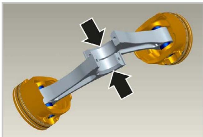
23 - When installing the connecting rods, check that the chamfers of the hole (motor shaft fixing) are opposite each other.
