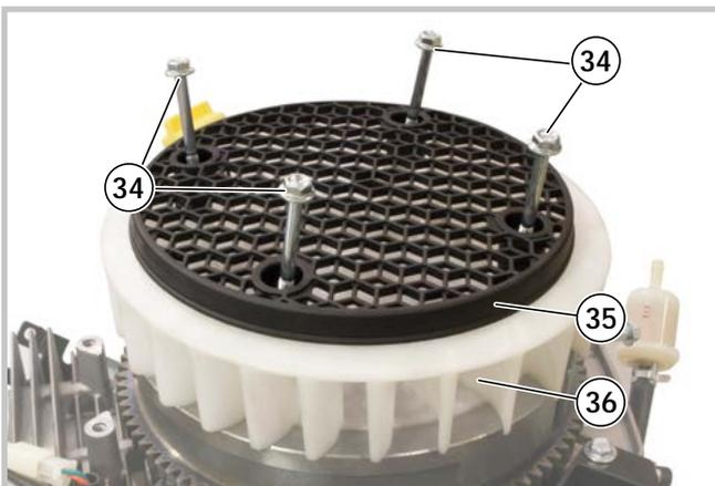
3 - Unscrew the four screws (34) and remove the grille (35) located above the fan (36).
