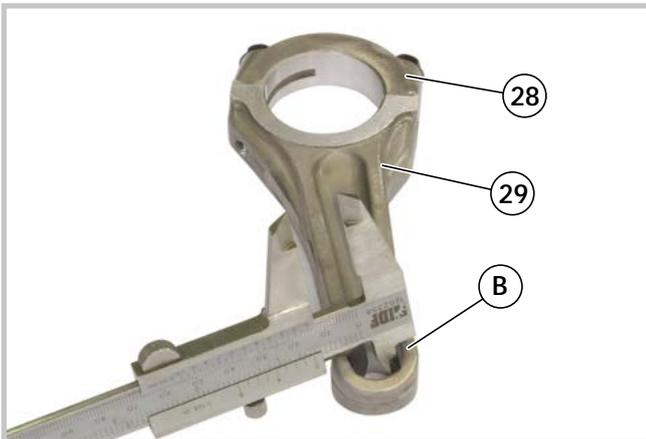
18 - Fit the cap (28) to the connecting rod (29) and check the diameter from the gudgeon pin side and the crank side; replace the connecting rod if the values are greater than:
