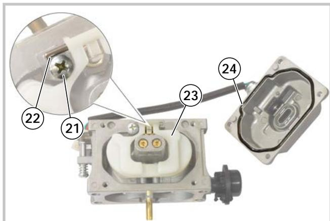
11 - Loosen the screw (21), remove the pin (22) from its housing and remove the float (23).
