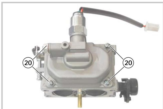
10 - Open the carburettor by unscrewing the four screws (20) on the tank (19).
