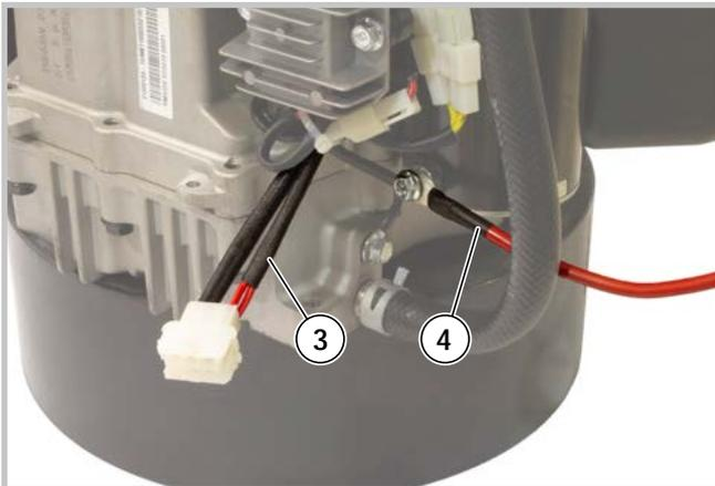
2 - Disconnect the connector (3) of the electrical cabling, the power supply cable (4) of the starting motor and the petrol pipe.
