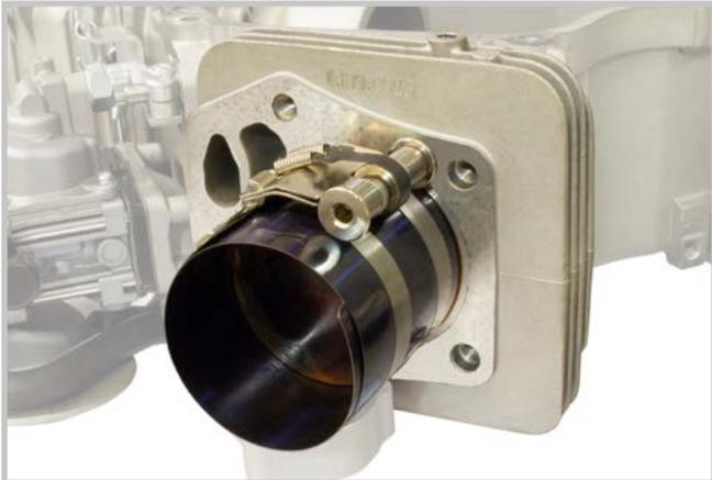
26 - Oil the inside of the piston liberally and insert the piston, with the marking facing the exhaust.
