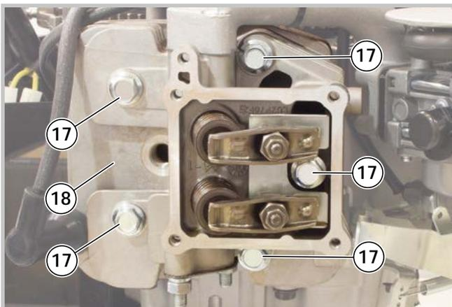
4 - Unscrew the five screws (17) and remove the cylinder head (18).
