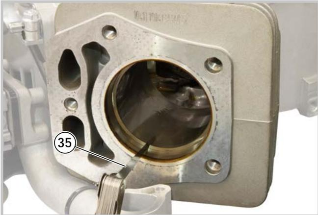
12 - To check the wear in the compression rings, insert them one at a time into the cylinder (32) by about 10-15 mm and measure the gap between the two ends with a feeler gauge (35); the rings must be replaced if the gap is more than 1,0 mm.
