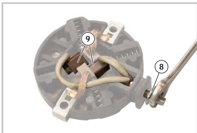
6 - Completely remove the nut (8) to remove the mass brushes (9) from the housing.
