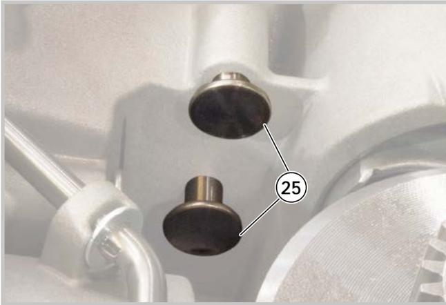
13 - Before fitting the camshaft ensure that the two tappets (25) are correctly housed in their seats.
