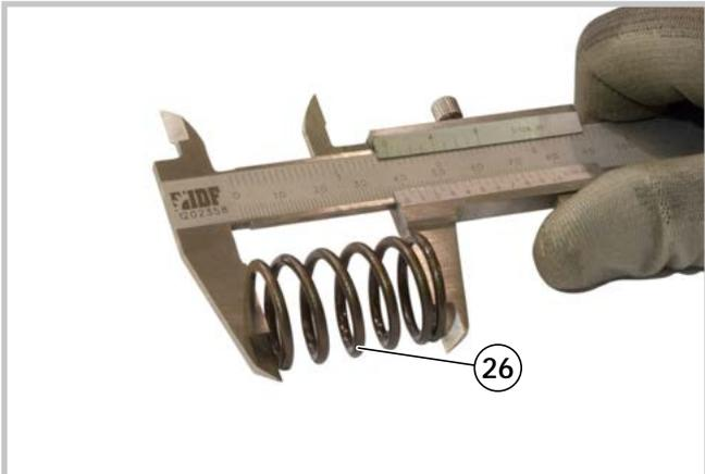
14 - Check the free length of the spring (26) and replace the spring if it is less than 39 mm.
