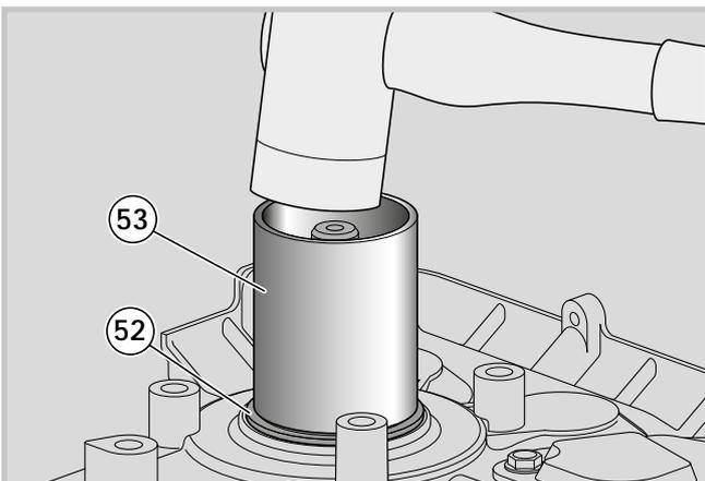
5 - The new ring (52) must be inserted with the help of a pipe (53) with a diameter of approximately 50-55 mm, taking care not to damage the sealing lip.
