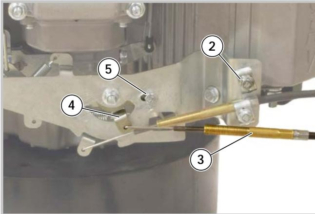
3 - Push the speed regulator lever (4) right until insert a plug (5) in the appropriate seat.
