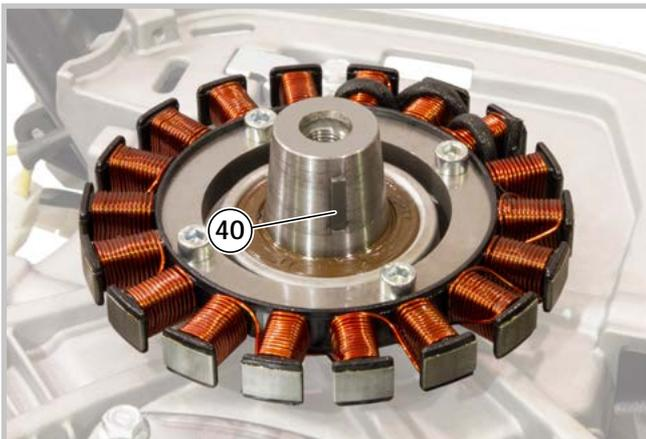
7 - Remount the coil (31) and (32) fixing the screws (33) to the indicated couple.
