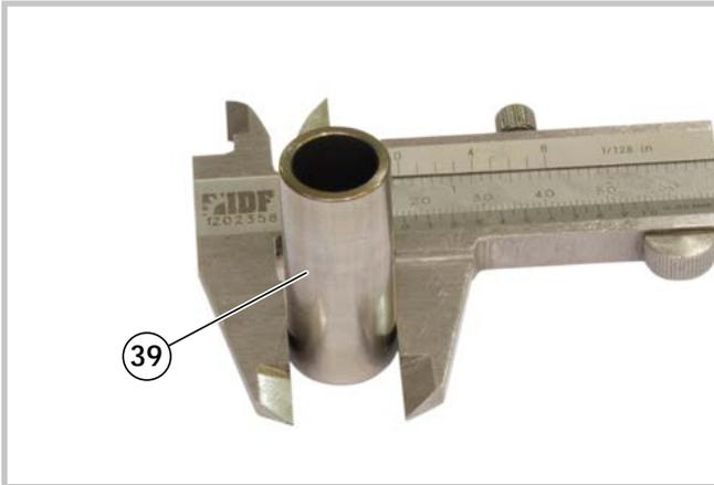
16 - Check the diameter of the gudgeon pin (39) in several places and replace it if it is less than 16,90 mm, even at a single point.
