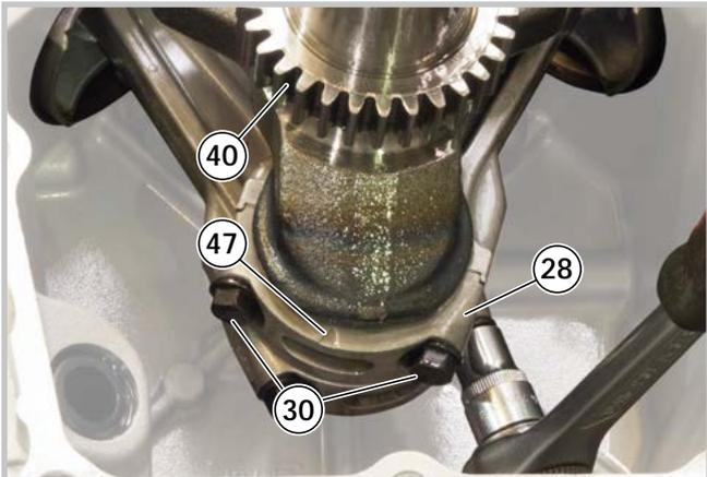
27 - Mount the engine shaft (40) and the connecting rod cap (28) with the relative screws (30), taking care with the position references (47) so as to avoid inverting the mounting direction of the cap.
