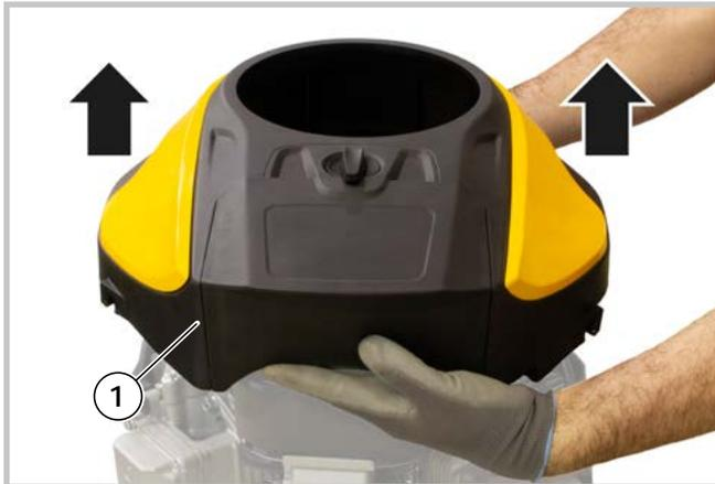
2 - Remove the cowl (1) from the engine by lifting it up.
