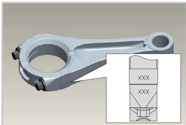
24 - The body of the connecting rod and the cap have the same order number, stamped on one side.
