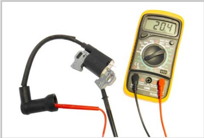
8 - Insert the tester terminal and remove the high voltage of the wire spark plug cap in contact with the iron wire and measure the resistance of the secondary coil. The resistance value must be between 18,2 and 21,2  $\Omega$ .
