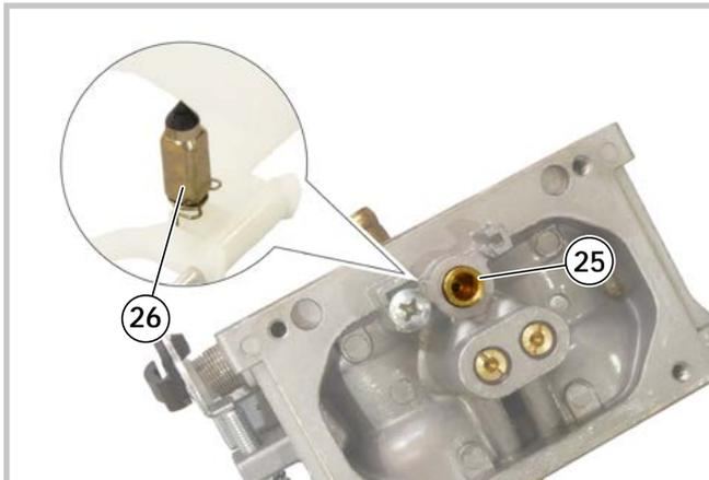
12 - Check that no impurities or dirt are deposited in the seat (25) of the needle (26).
