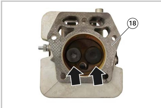
5 - Clean the cylinder head (18) and cylinder surfaces (19).
