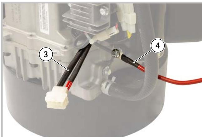
3 - Disconnect the two connectors (3) and (4) from the machine.
