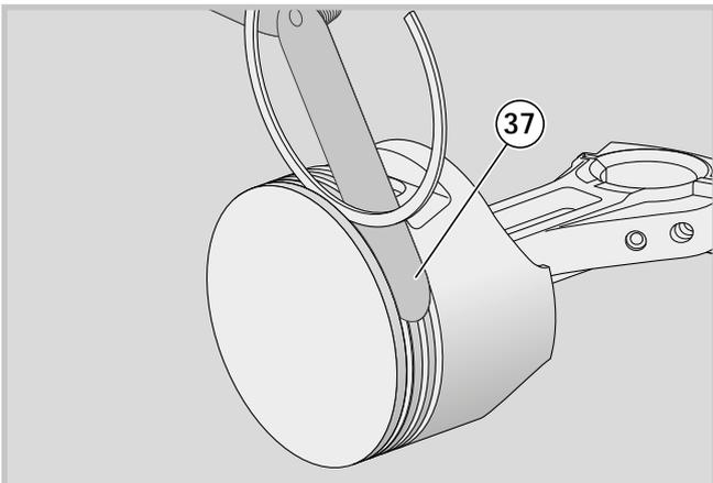
14 - To check the wear in the piston ring housings, fit a new ring and measure the residual space with a feeler gauge (37). The piston must be replaced if it is greater than 0,11 mm in the two compression ring housings.
