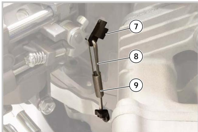
4 - Release the locking clip (7), remove the tie rod (8) of the "CHOKE" lever from its housing and the spring (9).
