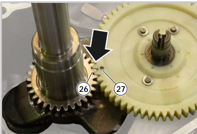
28 - After having fixed the connecting rod cap, take the greatest care to ensure that the two position references (26) and (27) punched on the engine shaft and camshaft gears, coincide, ensuring the correct distribution phasing.
