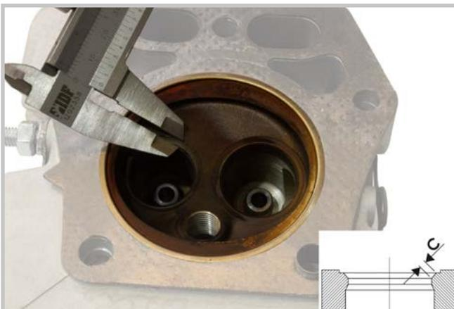
10 - Use a caliper gauge to check the width of the valve seat (C), which must be 2,0 mm; the cylinder head must be replaced if a greater value is measured.
