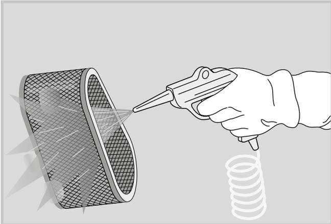
4 - Touch the cartridge on a solid surface and blow with compressed air from the interior side to remove dust and product residues.
