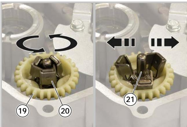
7 - Check that the irregular centrifugal (19) that are not present ruptures of the lubrication pallets.
