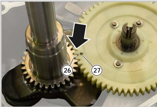
14 - When refitting the camshaft, maximum care must be taken to match up the two references (26) and (27) punched on the gears, so as to ensure correct distribution phasing.
