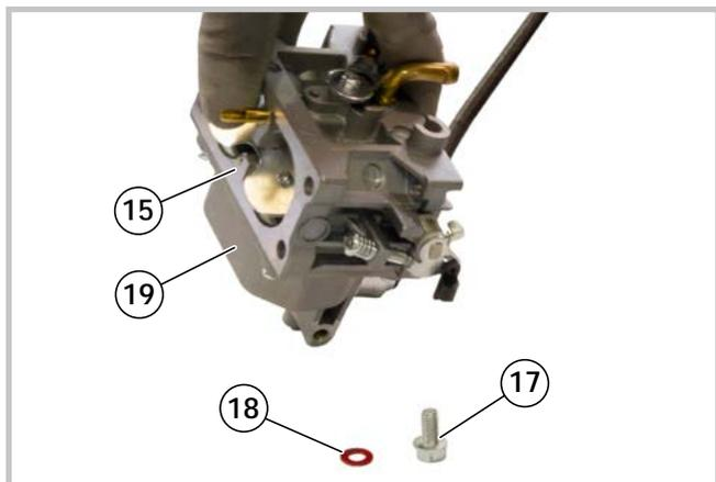
9 - Remove the screw (17), the washer (18) and by turning the carburettor (15), completely empty the petrol present in the tank (19) into a suitable container.
