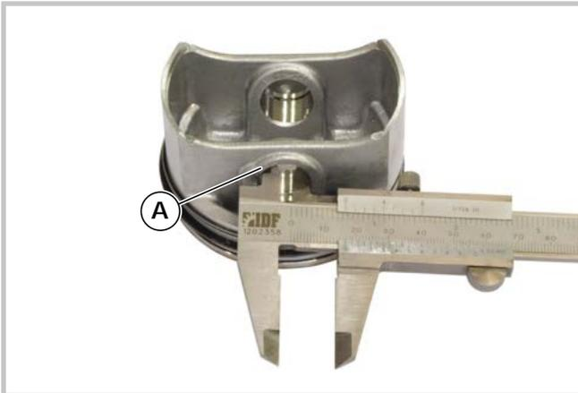
17 - Check the diameters of the gudgeon pin housings (A) on the piston (31) and replace the piston if they are more than 17,07 mm, even at a single point.
