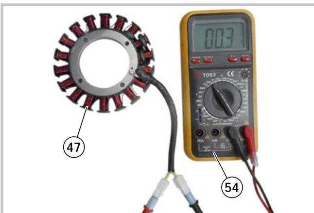
3 - Attach an appropriate tester (ohmmeter) (54) onto the alternator connectors (47). The value should be between 0,3 and 0,4  $\Omega$ .
