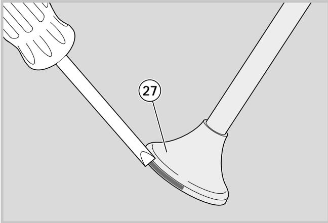
11 - Apply abrasive paste for grinding around the rim of the valve head (27) and then insert the valve into its seat.
