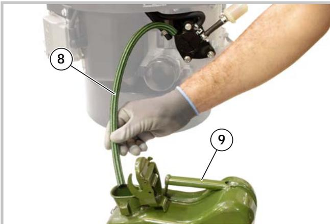
3 - Insert a tube (8) connected to an additional tank (9) and start the engine.
