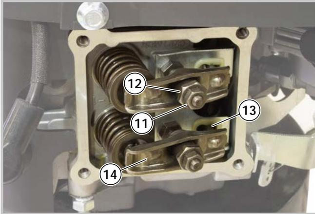
7 - The gap is adjusted by slackening off the nut (11) and suitably adjusting the register nut (12) until the above condition is reached.
