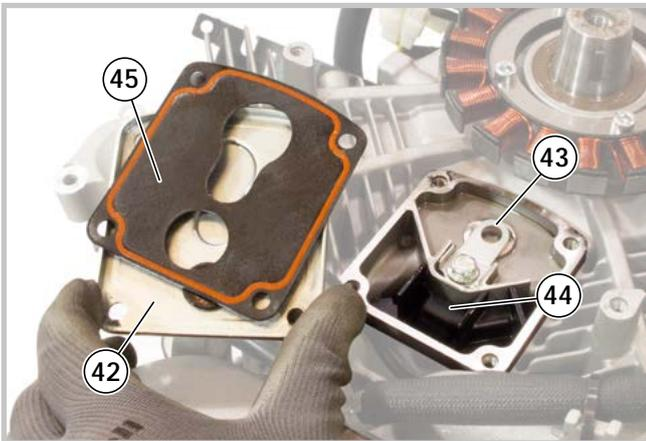
3 - Check that the lamella (43) is not blocked or deformed and check the status of the filter (44). Replace them if necessary.
