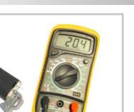
8 - Insert the tester terminal and remove the high voltage of the wire spark plug cap in contact with the iron wire and measure the resistance of the secondary coil. The resistance value must be between 18,2 and 21,2  $\Omega$ .
