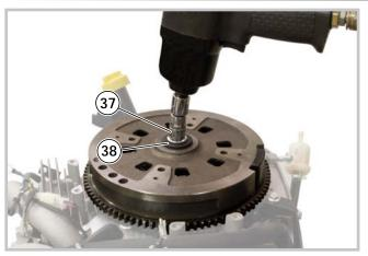
5 - Using a pneumatic gun, unscrew the nut (37) and recover the washer (38).
