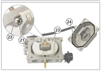
11 - Loosen the screw (21), remove the pin (22) from its housing and remove the float (23).
