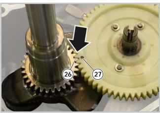
14 - When refitting the camshaft, maximum care must be taken to match up the two references (26) and (27) punched on the gears, so as to ensure correct distribution phasing.
