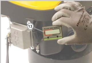
3 - Check the rotation speed on the speed indicator (13).
