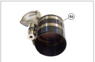
25 - Put the piston into the ring compression tool (46).
