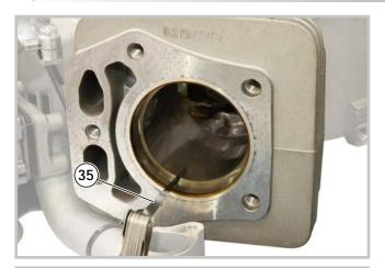
12 - To check the wear in the compression rings, insert them one at a time into the cylinder (32) by about 10-15 mm and measure the gap between the two ends with a feeler gauge (35); the rings must be replaced if the gap is more than 1,0 mm.
