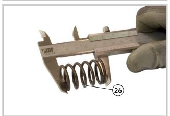
14 - Check the free length of the spring (26) and replace the spring of it is less than 39 mm.
