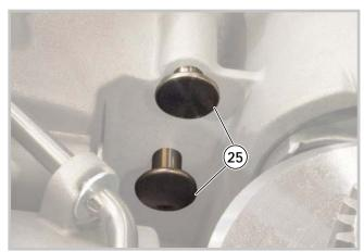
13 - Before fitting the camshaft ensure that the two tappets (25) are correctly housed in their seats.
