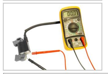
9.2. Adjusting the air gap and checking the coil
