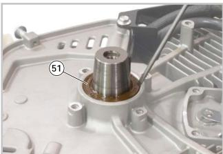
4 - Use a thin screwdriver inserted under the sealing lip to extract the oil seal ring (51).
