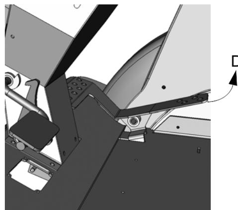
**Note** In cases where the cable is not sufficiently long to reach the maximum forward position on the pedal and on the pump the stop screw must be adjusted. At full speed forward the pedal must always be against the stop screw to prevent damage to the cable.
