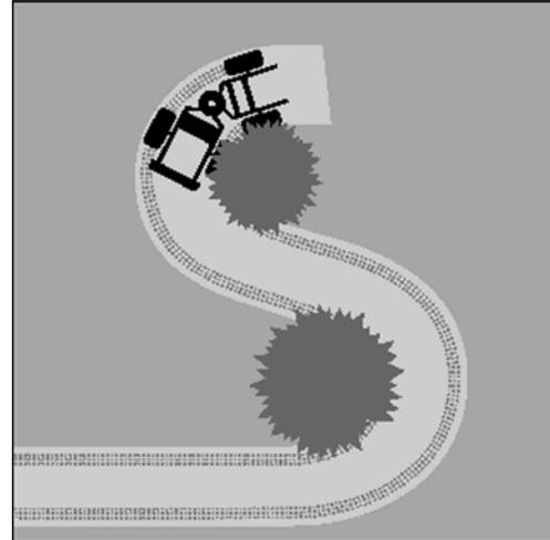
The articulated frame also pivots vertically,  $\pm 10^\circ$  when the machine is straight ahead and  $\pm 2^\circ$  at full lock. This makes it possible for all four wheels to press evenly against the ground when the machine is driven on uneven surfaces.
