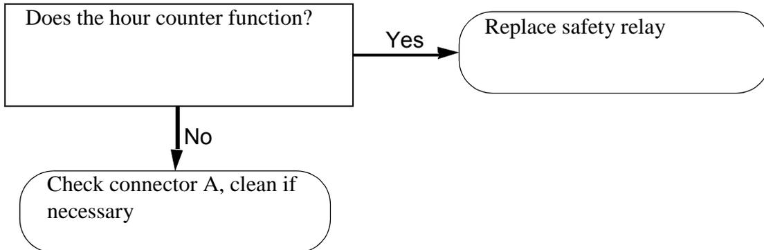
**6.2.9 The sand spreader does not function**
