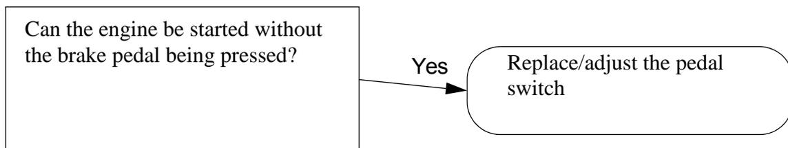
**6.2.8 The starter motor can be activated when the engine is running**
