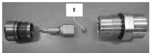
If after the ball replacement the problem is still unsolved, replace the complete check valve p/n 118830017/0 (F)
