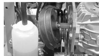
8. Remove the M10 screws G (3x) that hold the carrier plate/pulley to the flywheel as follows:
