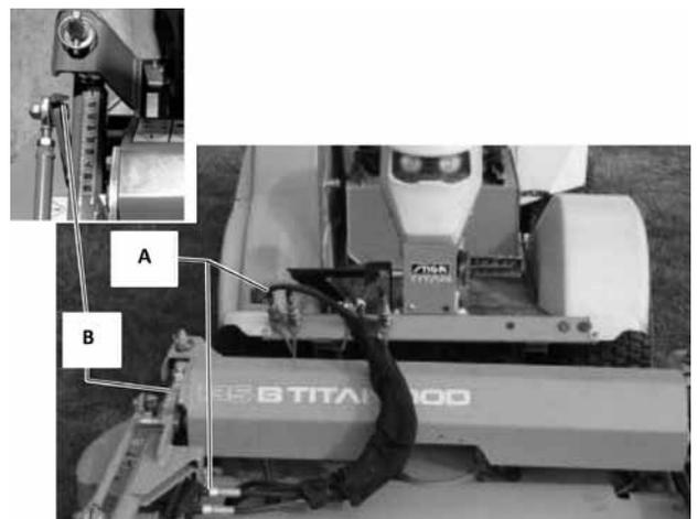
two hoses going to the cutting height cylinder.
