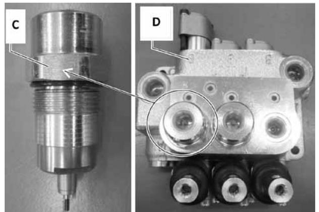
Open the check valve and replace the ball p/n 118830016/0 (E). Make sure the sealing area is well cleaned from debris.
