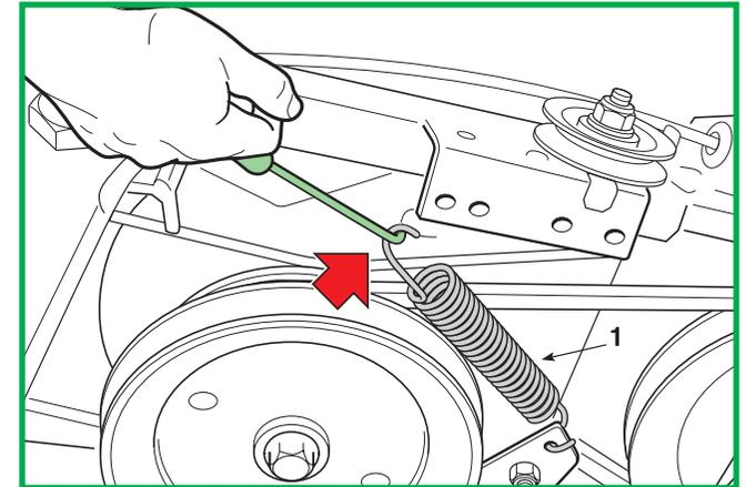
Unhook the drive belt tightener spring (1).
