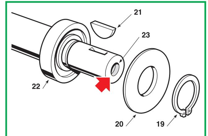
The second bearing still in place must be removed by hitting it from the inside of the flange using a 12 ÷ 15 mm diameter round bar (24).
