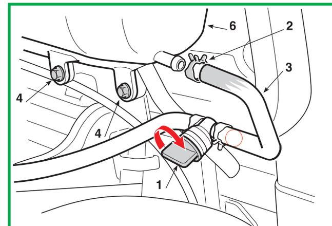
Unscrew the two lower screws (4) and the upper screw (5) fixing the tank (6) and remove the tank through the machine's right side.
