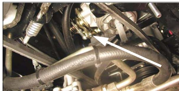
10. Place a collecting tray under the pump for collecting residual oil from the pump and hoses.
