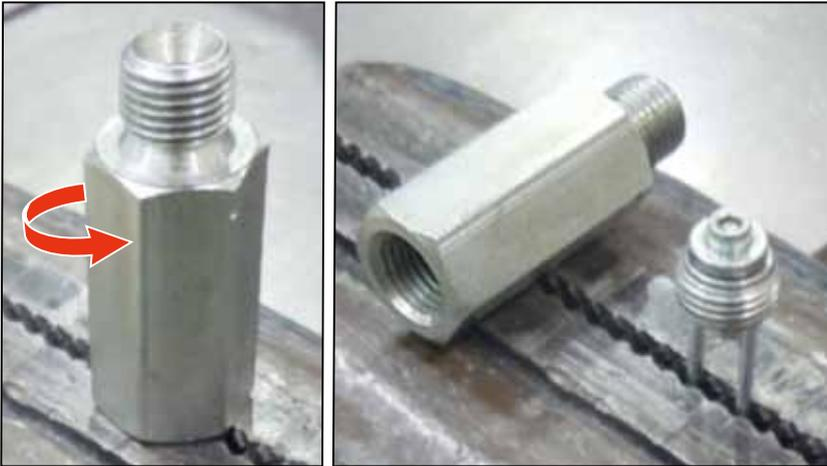
The dynamic balancing valve has a standard calibration of 0.15mm, this can be adjusted in the +/- 0.05 range compared to the standard calibration.
