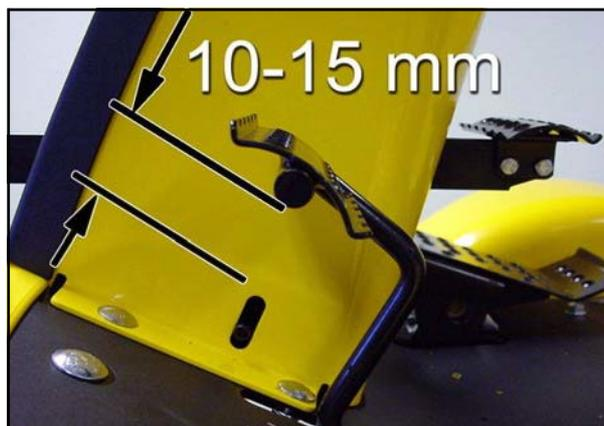
3. When the parking brake is activated the distance between the brake arm's rear stop and the brake arm should be 7-8 mm. *In the illustration the brake arm's return spring has been dismantled to make the picture more explicit.*
