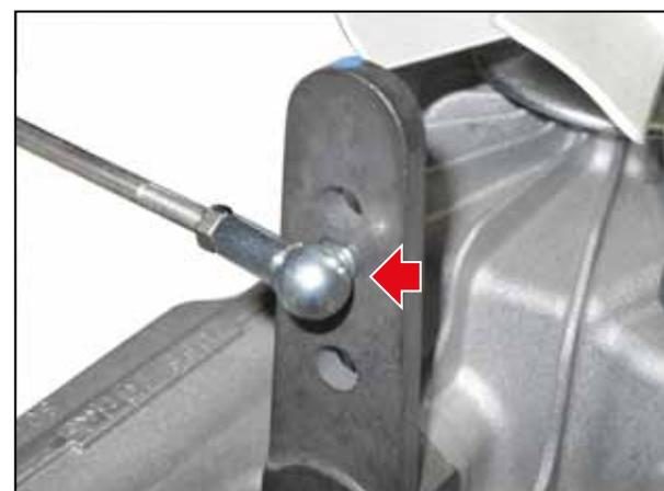
5. Check that the belt tensioner for the engagement of the deck functions correctly when the screw has been tightened, since the screw is also a link for the tensioning arm.
