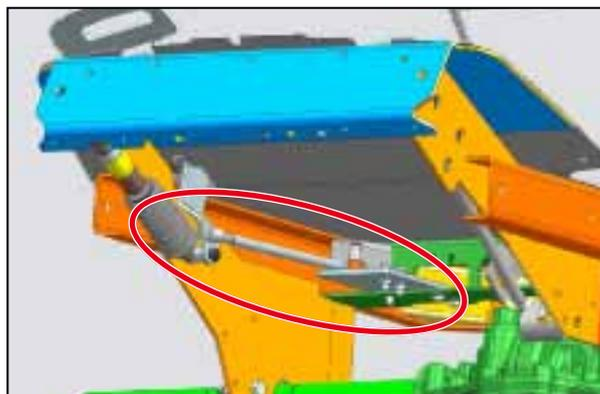
4. Fit the front and rear clamps. Make sure that the dogs at the clamps fit in the grooves in the wire cover. Both front and rear. See the figure.
