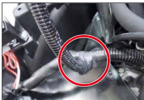
3. Place the main electric harness as closely as possible to the mudguard and pull the exceeding harness backwards as shown in the picture. This will avoid any possible contact with the battery case once mounted.
