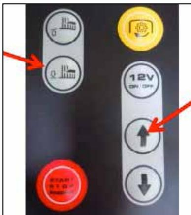
Push the button "HIGH GRASS DOWN" and "REAR RAKE UP" together, after urn ON the key and after 5 seconds in the display it will appear the message "TILT SAVED".
