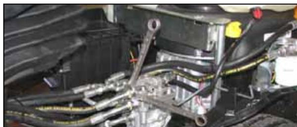
11. Remove the pump from the chassis by unscrewing the two M10 mounting nuts and screws. Use two 17 mm spanners. See the figure.
