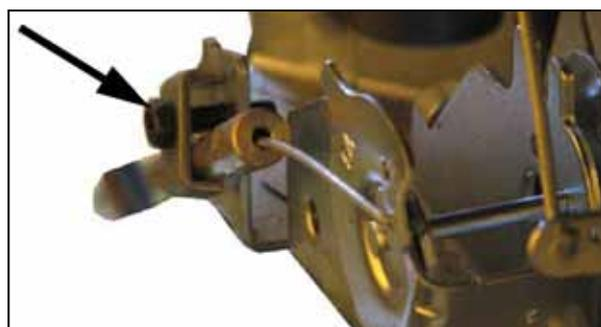
6. Push out the choke wire and the throttle wire from the holder at the articulating point.
