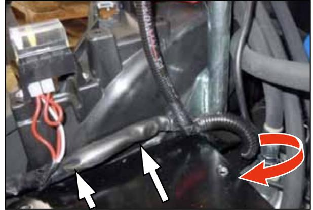
4. Secure the electric harness underneath the battery area by fastening the harness to the main frame bracket with a cable tie.
