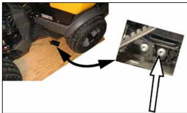
5. Unscrew the nut and unhook the spring. See the fig.
