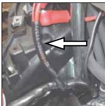
**IMPORTANT - Carefully check that the positive wires (red) are integral, that the insulation is not cracked or worn and that the corrugated protection sheath is installed and correctly mounted to prevent cables from being crushed by the battery housing after installation.**
