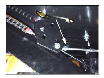
2. Release the upper nut on the stop screw and screw down the screw a few turns.
