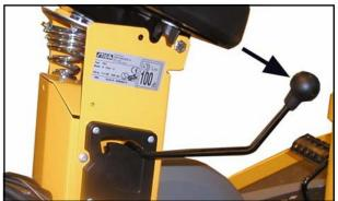
2. Disconnect the brake rod from the brake shoe arm.
