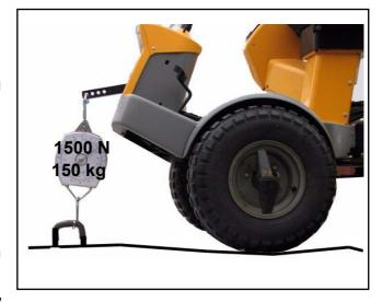
If the steering is comfortable when the screw is in its upper position and the lifting capacity is OK when the screw is in its lower position, replace the charge pump in the HST.
