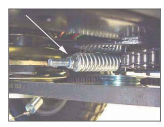
2. Loosen the screws that hold the pulley so that the wire can be taken out between the pulley and the wire retainer.
