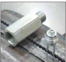
The dynamic balancing valve has a standard calibration of 0.15mm, this can be adjusted in the +/- 0.05 range compared to the standard calibration.
