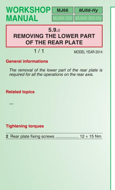
The lower part of the rear plate (1) is fixed to the upper part with 7 screws (2).
