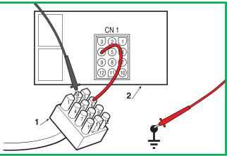
This operation must be done by making a bridge between contacts 6 (CN1) of the wiring connector (1) and the card connectors (2), so making contact with the ferrules of the electronic card (2). You should obtain the following result:
