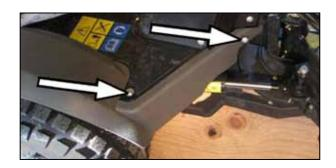
3. Unscrew one M6 nut from the under side and one screw and remove the left front art. cover.
