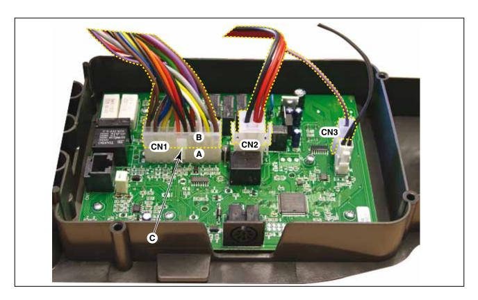
Note! The electronic card is connected to the system by means of connectors CN1,
