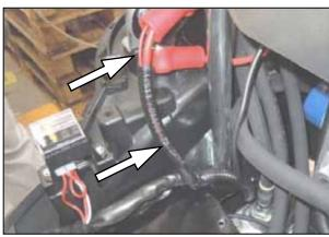
2. Secure the lower end of the corrugated sheath to the main harness with duct tape.
