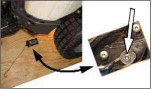
2. Unscrew one M6 nut from the under side and one screw and remove the left floor cover.
