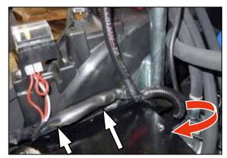
4. Secure the electric harness underneath the battery area by fastening the harness to the main frame bracket with a cable tie.
