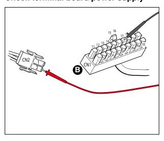
Set the tested in "voltmeter" mode (Volt DC0 - 20).
