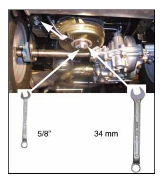
Note! Check that the dog fits in the hole in the magnetic clutch. See the figure.
