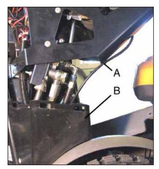
5. Loosen the nut at the rear of the engine and hook off the wire.
