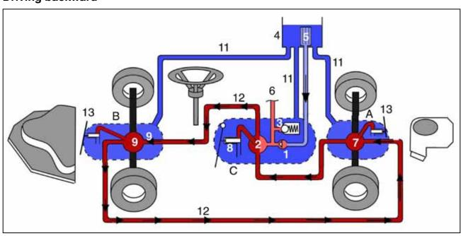
The charge pump (1) and the main pump (2) are integrated into one unit, the hydraulic pump (C) which is located separat in front of the engine.
