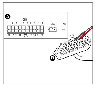
Set the tester in "ohmmeter" mode.
