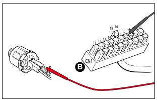
Set the tested in "voltmeter" mode (Volt DC0 - 20).
