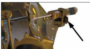
6. Push out the choke wire wire from the holder at the articulating point.
