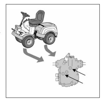
4. Check that the clutch release lever (R) is in the outer position (drive position).
