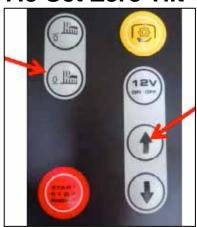
Push the button "HIGH GRASS DOWN" and "REAR RAKE UP" together, after urn ON the key and after 5 seconds in the display it will appear the message "TILT SAVED".
