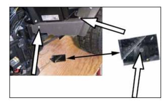
8. Check that the fuel cock is correct placed in the opening of the cover. See the figure.
