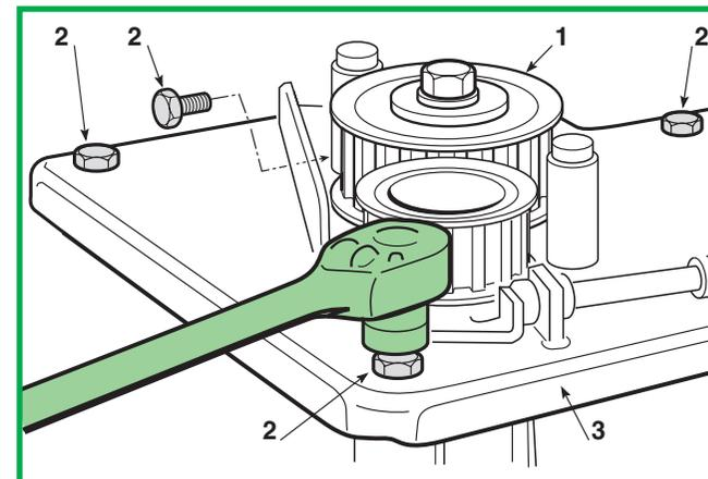
Extract the two toothed pulleys (1) from the blade shafts, undo the seven screws (2) fixing the plate (3) and remove it.
