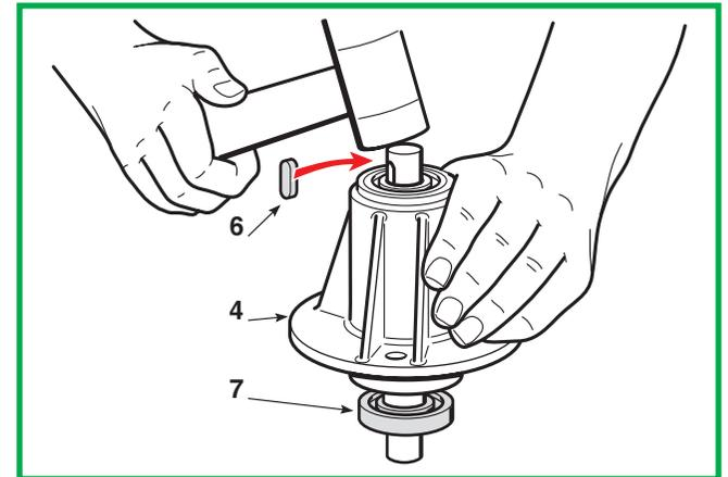
If only the shaft or bearings are to be replaced, remove the key or the two keys (6) and hit the shaft on the pulley side with a plastic mallet to extract the shaft together with the lower bearing (7).
