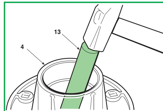
On reassembly, having first inserted the shaft in the lower bearing hole and inserted everything into the support, fit the upper bearing using the specific stopper (14) **that acts on the inner ring**, hitting it squarely with a mallet until the bearing is fully driven home.
