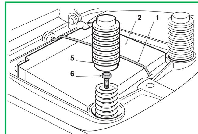
Remove the caps (5) from the springs and undo the screws inside (6).
