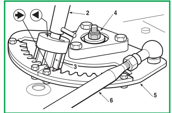
Toothed sectors (10) are secured to the ring gear (5) by screws and nuts (11).
