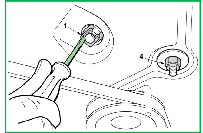
**A) Dismantling the steering pinion and ring gear**
