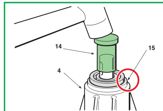
When refitting the plate (3), **the holes corresponding to the support axes must meet perfectly in the centring step (15)** cut into the upper part of each support.
