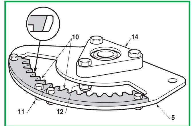
Check ring gear allowance (5) compared to the pin (12); if excessive, replace the bearing.
