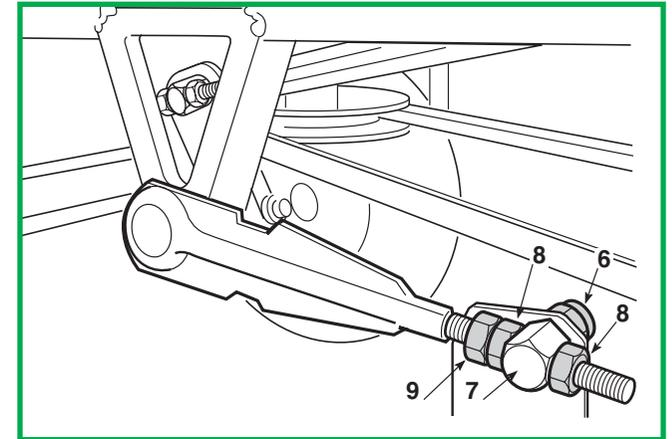
On reassembly ensure that the two rear holes of the corner joints are used for fixing the pins (7), without locking the relative nuts (6).
