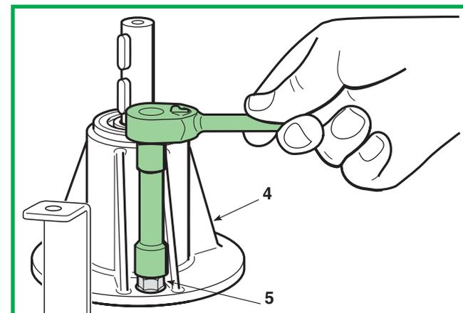
Dismantle the flanged support (4) by unscrewing the three fixing screws (5).
