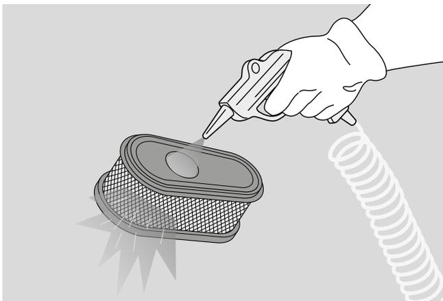
5 - Beat the cartridge on a solid surface and blow with compressed air from the interior side to remove dust and product residues.
