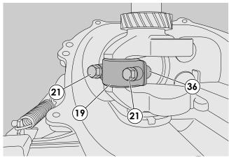
23 - Mount the engine shaft (24) and the connecting rod cap (19) with the relative screws (21), taking care with the position references (36) so as to avoid inverting the mounting direction of the cap.
