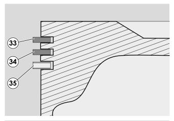
19 - To refit the rings to the piston, first fit the three oil scraper rings (33), then the ring with a round edge (34) and finally the ring with a sharp edge (35), being careful over the markings (which must face the piston head) and in arranging the gaps to ensure that they are not aligned with each other;
