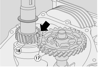
12 - When refitting the camshaft, maximum care must be taken to match up the two references (17) and (18) punched on the gears, so as to ensure correct distribution phasing.
