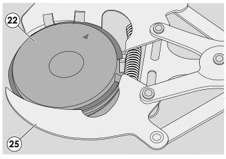
15.3. Dismantling and checking the piston, piston rings, connecting rod and engine shaft
