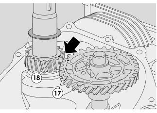
24 - After having fixed the connecting rod cap, take the greatest care to ensure that the two position references (17) and (18) punched on the engine shaft and camshaft gears, coincide, ensuring the correct distribution phasing.
