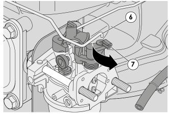
6 - Remove the tie rod (6) of the AUTO-CHOKE lever by releasing the locking clip (7). Slightly pull out the carburettor to facilitate the release of the intake butterfly shaft.
