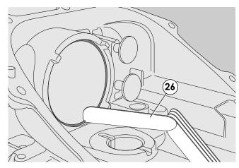
10 - To check the wear in the compression rings, insert them one at a time into the cylinder (23) by about 10-15 mm and measure the gap between the two ends with a feeler gauge (26); the rings must be replaced if the gap is more than 1,0 mm.
