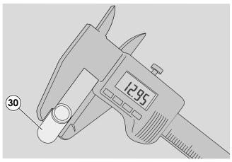
14 - Check the diameter of the gudgeon pin (**30**) in several places and replace it if it is less than 12.95 mm, even at a single point.
