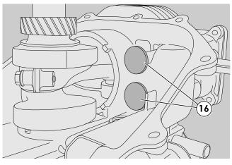
11 - Before fitting the camshaft ensure that the two tappets (16) are correctly housed in their seats.
