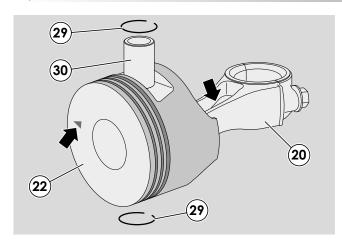
20 - Fit the connecting rod (20), gudgeon pin (30) and clamping rings (29) to the piston (22).
