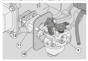
8 - Completely remove the carburettor (9) the gasket (10), the spacer (11) and the heat protection gasket (12).
