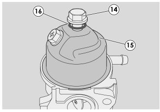
9 - Unscrew the central screw (14) securing the tank (15) and remove the corresponding OR (16).
