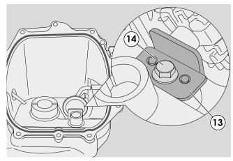
9 - In the case of breakage or irregular operation of the counterweights the whole group, fixed by a plate (13) and a screw (14) must be replaced.
