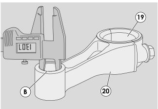
16 - Fit the cap (19) to the connecting rod (20) and check the diameter from the gudgeon pin side and the crank side; replace the connecting rod if the values are greater than:
