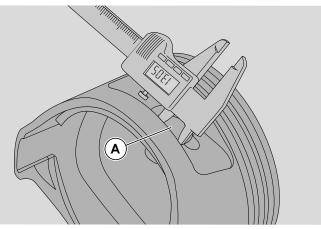
15 - Check the diameters of the gudgeon pin housings (A) on the piston (22) and replace the piston if they are more than 13.05 mm, even at a single point.
