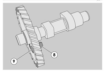
6 - Check the regular movement of the pressure reducer (8) and the efficiency of the spring (9); the whole group must always be replaced in the case of breakage or irregular operation of the pressure reducer.
