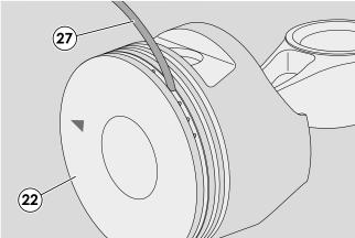
11 - Use a section of an old ring (27) to carefully clean the inside of the piston (22) ring housings, ensuring that the oil passage holes are not blocked.
