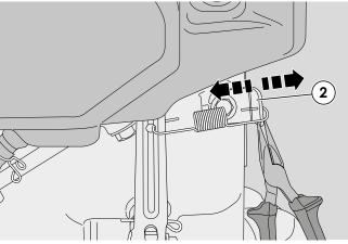
2 - Using pliers, bend the plate (2) slightly to the right to increase the number of revs and to the left to reduce them.
