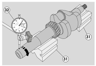
18 - To check the alignment between the manifolds and the protruding part of the shaft, place the engine shaft on two prismatic guides (31) and, with the help of a comparator (32) placed at the end, check the displacement by rotating the shaft. The shaft must be replaced if the displacement exceeds 0.10 mm.
