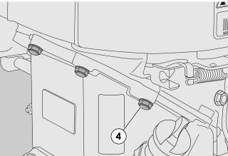
25 - Close the carter and fix the screws (4) to the indicated couple [  $\stackrel{\frown}{\text{[[]}}$  15.1].
