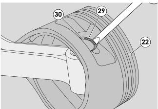
13 - Use a screwdriver to remove the clamping ring (29) and remove the gudgeon pin (30) from the piston (22).
