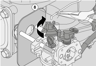
7 - Rotate the butterfly valve clockwise 90° and, using pliers, disconnect the intake butterfly rod (8).
