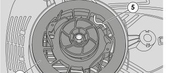
3 - Undo or cut the knot at the end of the rope (5) and remove the section still attached to the pulley.
