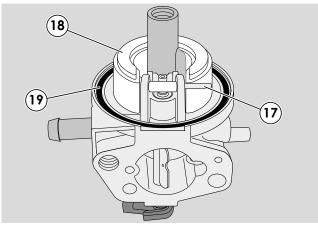
10 - Pull out the pin (17), dismount the float (18) and remove the gasket (19).
