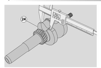
17 - On the engine shaft (24), removed beforehand, use a digital gauge to check the diameter of the connecting rod pin.
