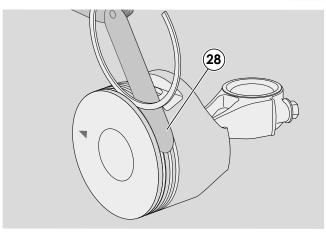
12 - To check the wear in the piston ring housings, fit a new ring and measure the residual space with a feeler gauge (28). The piston must be replaced if it is greater than 0.15 mm in the two compression ring housings.
