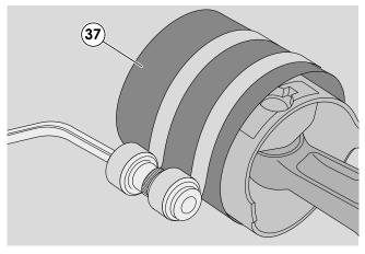
22 - Oil the inside of the piston liberally and insert the piston, with the marking facing the exhaust.
