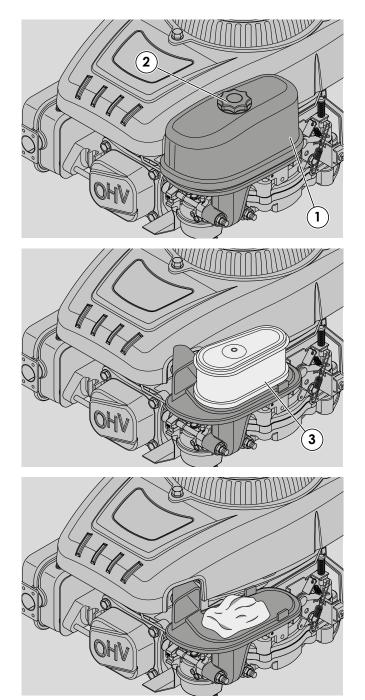
7.1. Maintenance of filtering element
