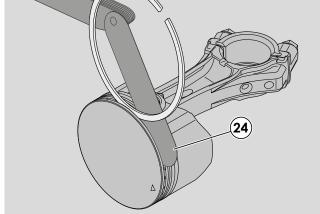
9 - Use a section of an old ring (23) to carefully clean the inside of the piston (19) ring housings, ensuring that the oil passage holes are not blocked.
