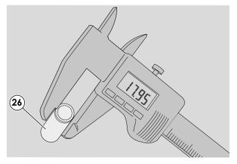
12 - Check the diameter of the gudgeon pin (**26**) in several places and replace it if it is less than 17,95 mm, even at a single point.
