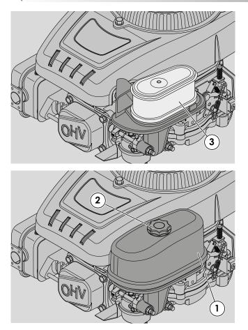
9 - Reassemble in their seats the filter element (3) and its cover plate (1) by turning the dedicated knob (2).
