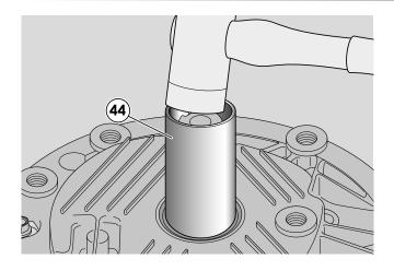
4 - Complete the insertion with the help of a pipe(44) of a diameter of approximately 30-35 mm.
