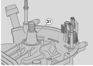
14.5. Dismantling and replacing the magneto flywheel
