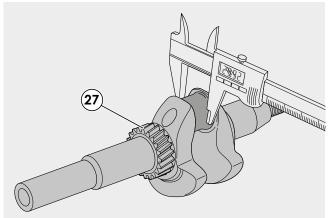
15 - Remove the engine shaft (27) checking the diameter of the connecting rod pin with a digital gauge.
