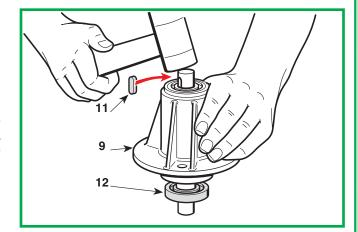
After having removed the snap ring (13), the dust cover (14) and the spline (15), the bearing (12) splined onto the shaft can be removed using a normal extractor, taking care to close up the threaded hole (16) with a screw to prevent the point of the extractor from damaging the thread.
