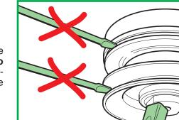
IMPORTANT - To remove the clutch (2) from the engine shaft, absolutely do not use a lever to force the pulleys or the outer cover. In case of difficulty, apply an unlocking spray and gently tap on the hub with a hammer, to facilitate extraction.
