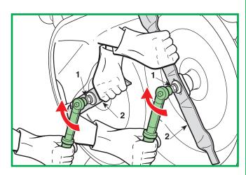
4.9.0 **REMOVING, SHARPENING** AND BALANCING THE BLADES
