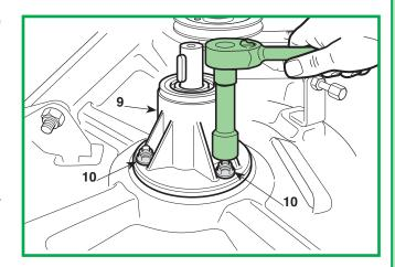
If you should want to just replace the shaft or bearings, remove the key (11) and hit the shaft with a plastic mallet on the pulley side in order to remove the shaft together with the lower bearing (12).
