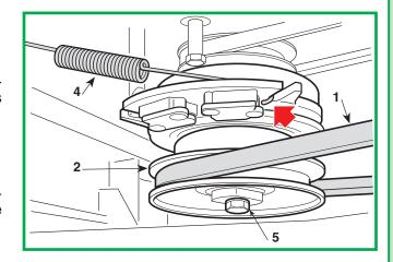
Free the blade belt (1) from the clutch pulley (2).
