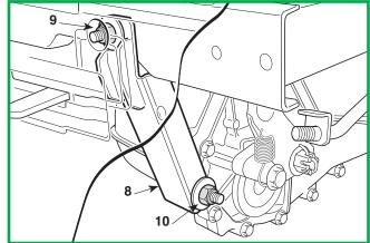
5.6a.0 REMOVAL OF THE REAR AXLE Hydro-Gear T2-ADBF-2X3C-1RX1
