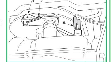
Remove the split pin (7) and disconnect the gear control rod (8).
