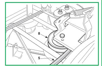
Loosen the nut (7) for the drive pulley (8) to the point where the passage of the belt is allowed (5).
