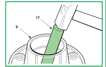
On reassembling, first put the shaft into the hole of the lower bearing and insert this into the support. Fit on the upper bearing and, using the special bush (18) **which works on the inner ring**, hit it squarely with a mallet until the bearing is fully driven home.
