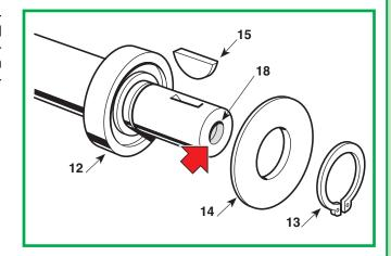
The second bearing still in place must be removed by hitting it from the inside of the flange using a  $12 \div 15$  mm diameter round bar (17).
