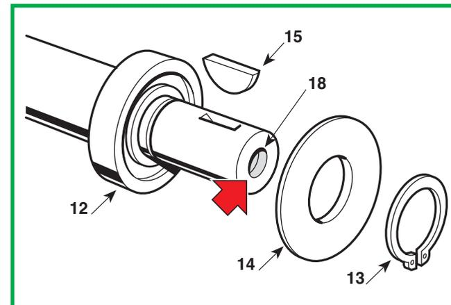
The second bearing still in place must be removed by hitting it from the inside of the flange using a 12 ÷ 15 mm diameter round bar (17).
