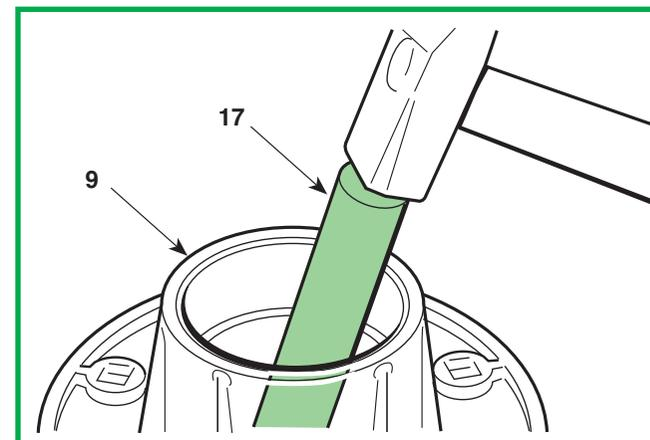
On reassembling, first put the shaft into the hole of the lower bearing and insert this into the support. Fit on the upper bearing and, using the special bush (18) **which works on the inner ring**, hit it squarely with a mallet until the bearing is fully driven home.
