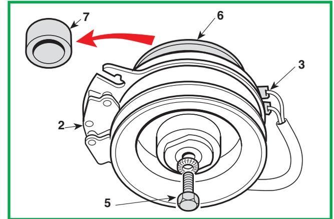
Disconnect the connectors (3) from the clutch contacts (2), unhook the return spring (4) from the clutch side and unscrew the central screw (5) with the help of a power screwdriver.
