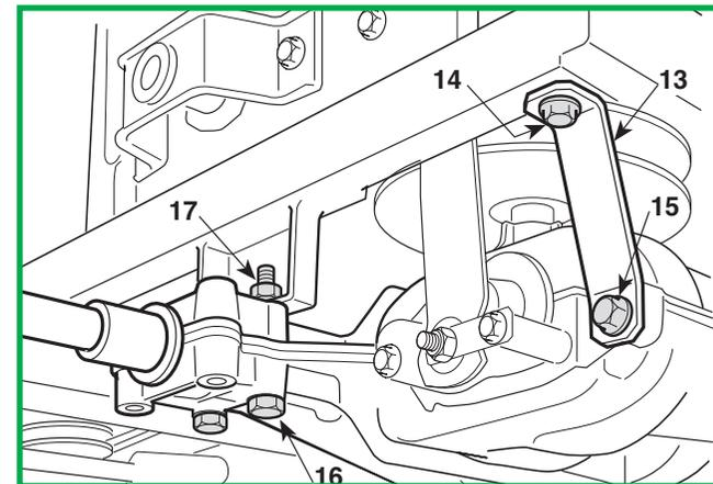
Loosen the screw (14) to give a minimum of movement to the bracket (13) and undo the two screws (16). Then carefully loosen the four nuts (17), holding up the unit so that it does not fall.
