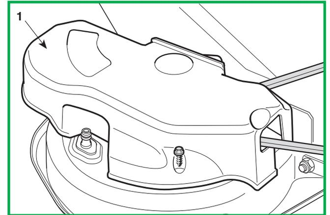
When reassembling the right (1) and left (2) guards, keep the belt (3) taut so that it is well-inserted in the pulley grooves and do not interfere with the belt guides inside the guards.
