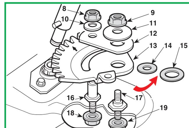
Check pin (16) and (17) wear and, if necessary replace them by unscrewing the relevant nuts (18) and (19).
