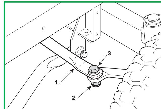
Toe-in check may only change due to rod deformation (1) or due to spindle bushing wear.
