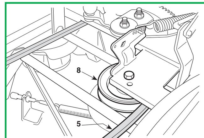
Hold the two parts of the belt (5) to release it from the pulley (6).
