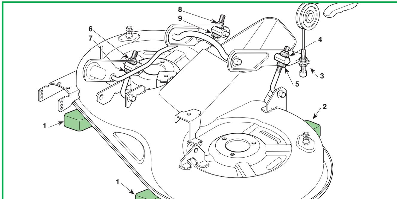
Turn the adjuster (3) until the control cable is taut. Tighten the two right upper nuts (6 - 8) and the left upper nut (4) to the point where the deck just begins to lift, then tighten the three locknuts (5 - 7 - 9).
