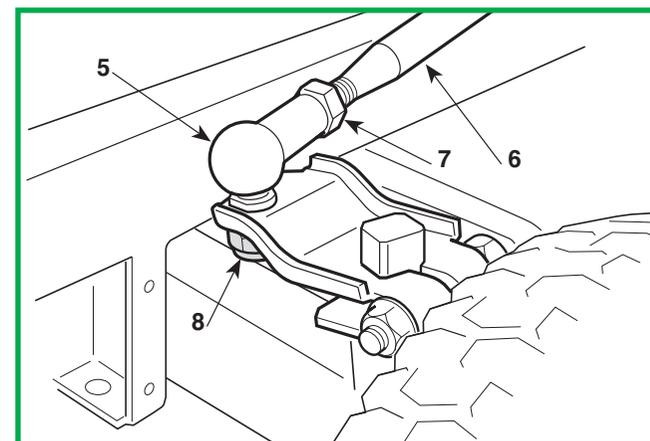
If the steering wheel is not straight, dismantle the articulated joint (5) and screw down or up on the tie-rod (6) for the necessary amount.
