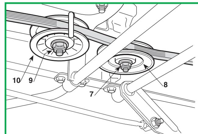
Unscrew the nut (9) and take off the pulley of the guide pulley (10).
