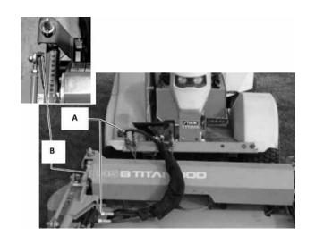
two hoses going to the cutting height cylinder.
