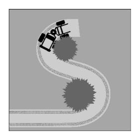
The articulated frame also pivots vertically, ±10° when the machine is straight ahead and ±2° at full lock. This makes it possible for all four wheels to press evenly against the ground when the machine is driven on uneven surfaces.
