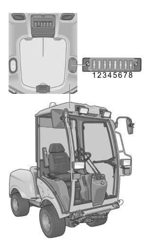
Two fuse boxes are located in accordance with the figure to the right. These contain the fuses according to the table below:
